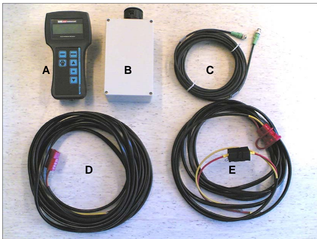
Fig. 1: The parts for the Control Automation System (the control unit A in the picture lacks a control facility for the driveline marker)
