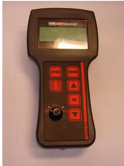
Fig. 2: This is a newer Tassu equipped with the driveline marker facility.
