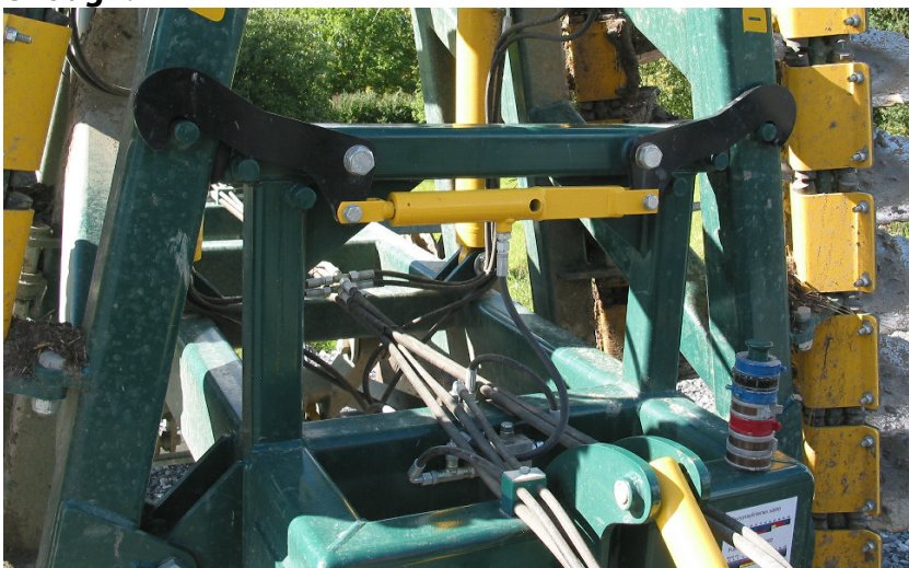
Figure 1. Wing section lock mechanism
