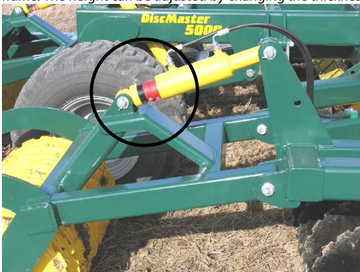
Figure 4 Adjusting cultivation depth
