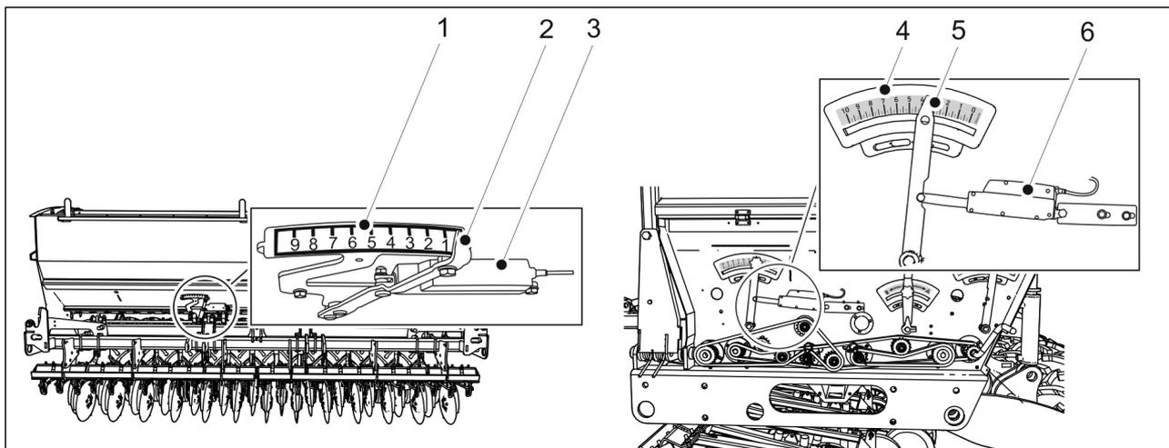
**Figure. 4.2.1.8. - 22. Linear actuator for remote control. On the left, a machine without a gearbox and, on the right, a machine equipped with a gearbox on the seed side. On the right, a machine with a dual gearbox.**
