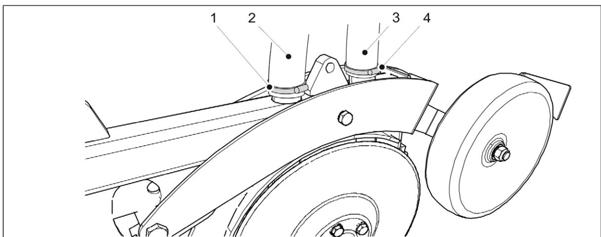
**Figure. 7.9.1.1. - 245. Disconnecting coulter hoses**
