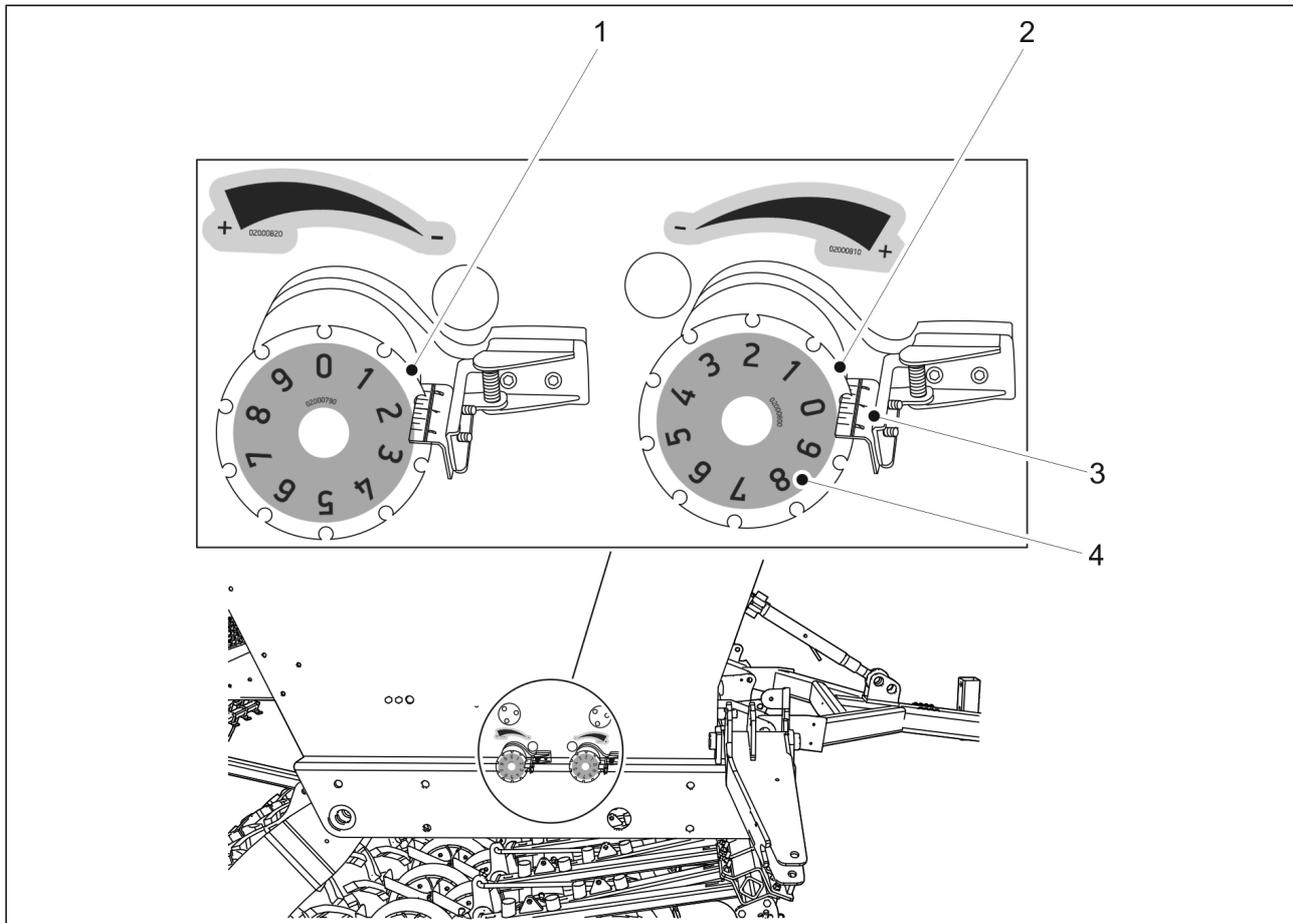
**Figure. 6.6.5. - 120. Adjusting the width of the feeder roller**
