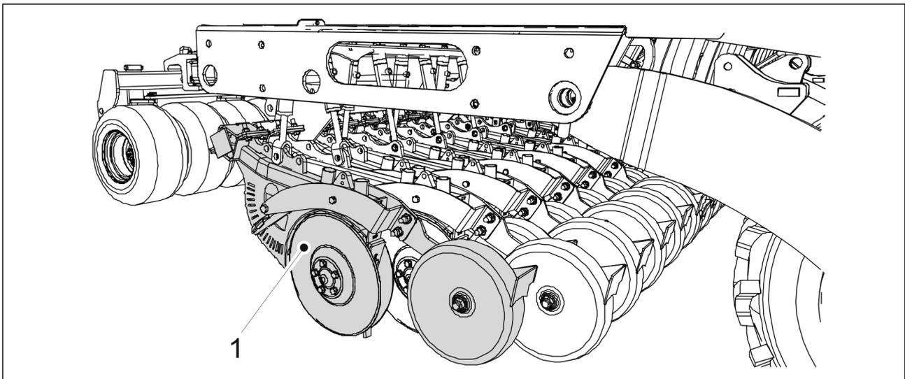
**Figure. 7.9.1.1. - 244. Lowering coulters to the ground**
