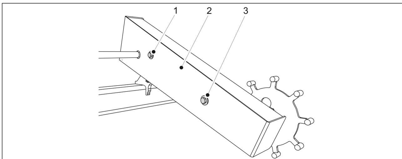
**Figure. 7.1.6. - 185. Cover of the wheel drive housing**
