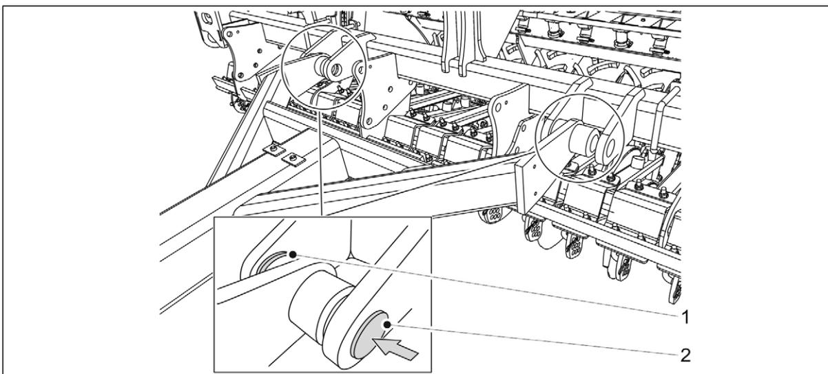
**Figure. 5.1.1. - 52. Mounting the wheel packer**
