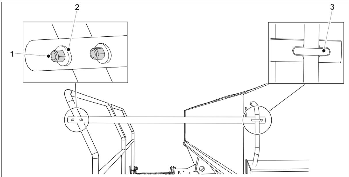
**Figure. 5.1.10. - 71. Attaching the end railing of the working platform**
