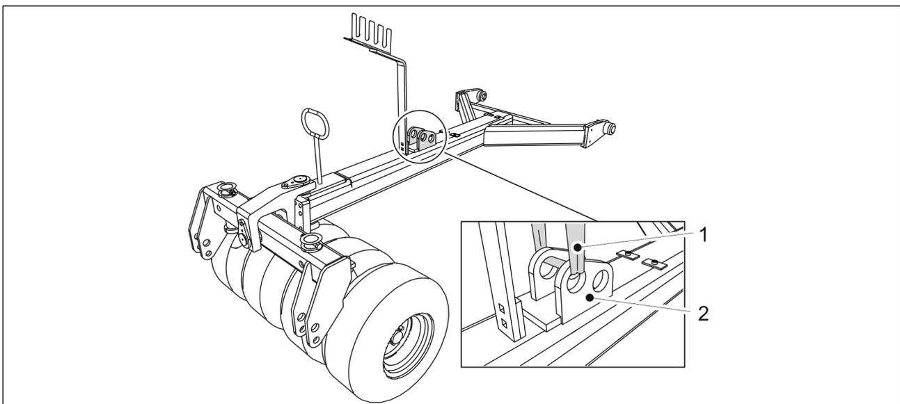
**Figure. 5.1.1. - 51. Lifting the wheel packer**
