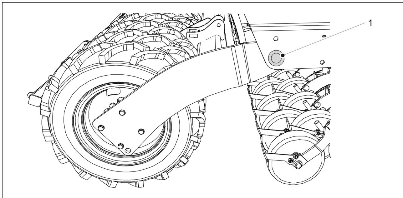
**Figure. 7.2.4. - 200. Rear axle mounting**
