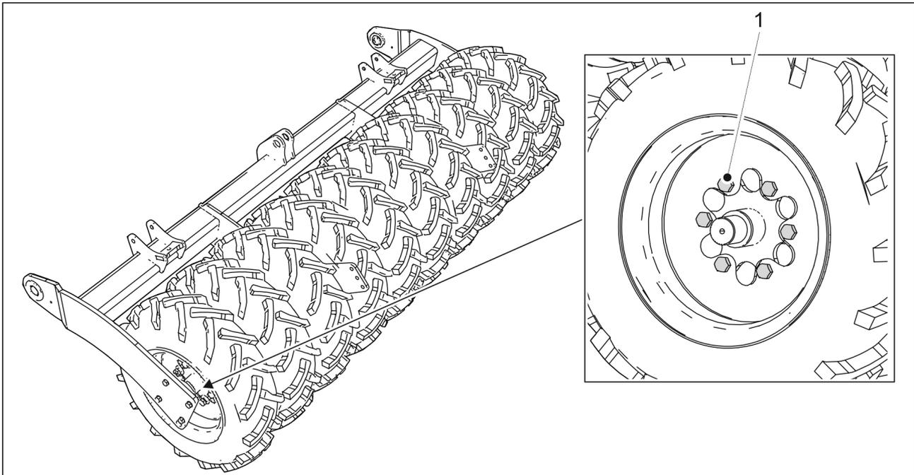
**Figure. 7.1.2.1. - 171. Wheel bolts of the transport wheels**
