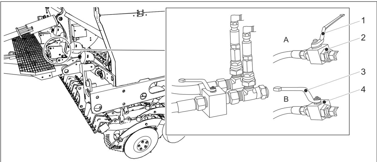
**Figure. 5.3.5. - 89. Lifting circuit ball valves**
