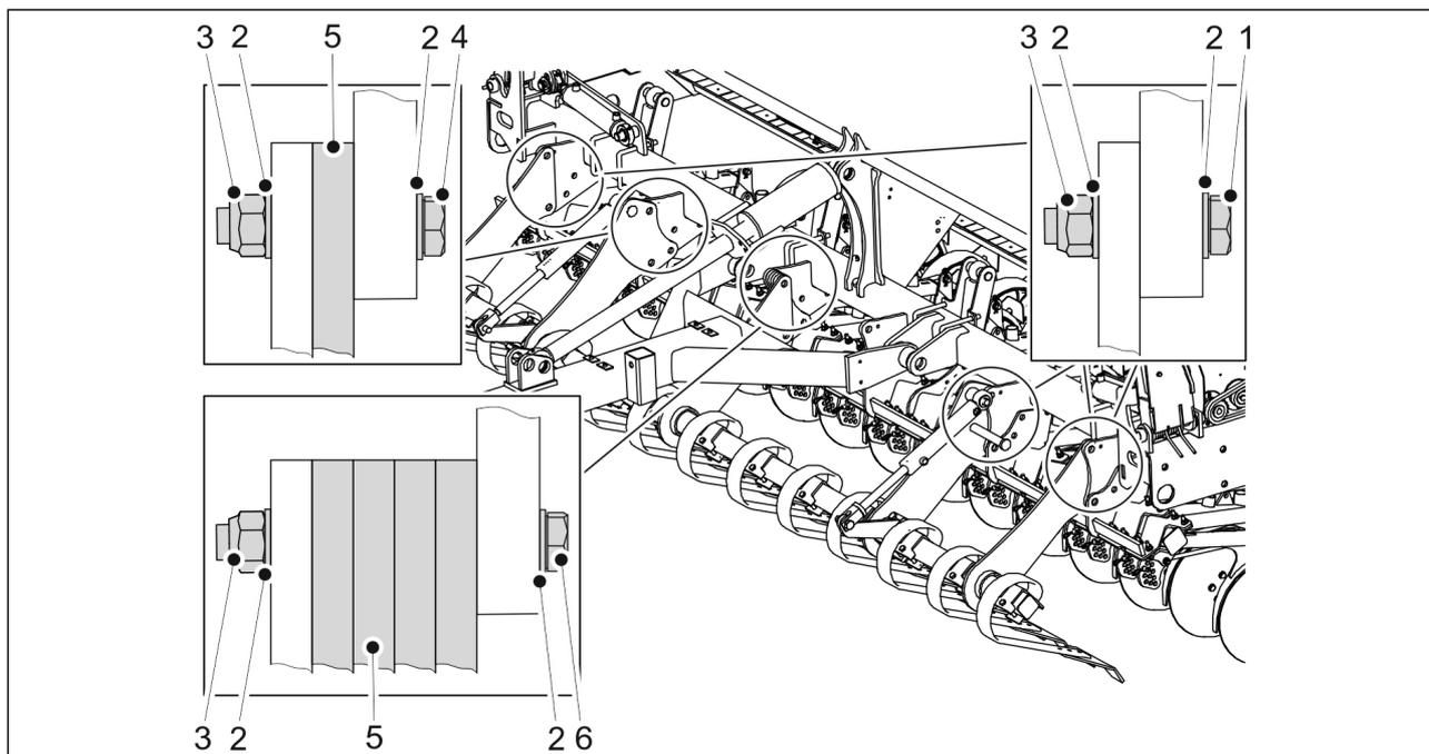
**Figure. 5.1.4. - 59. Mounting the front levelling board on a FX400**
