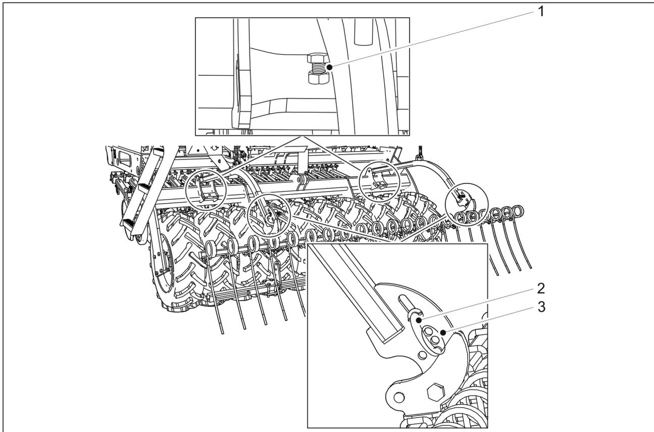
**Figure. 6.11. - 163. Adjusting the rear harrow**
