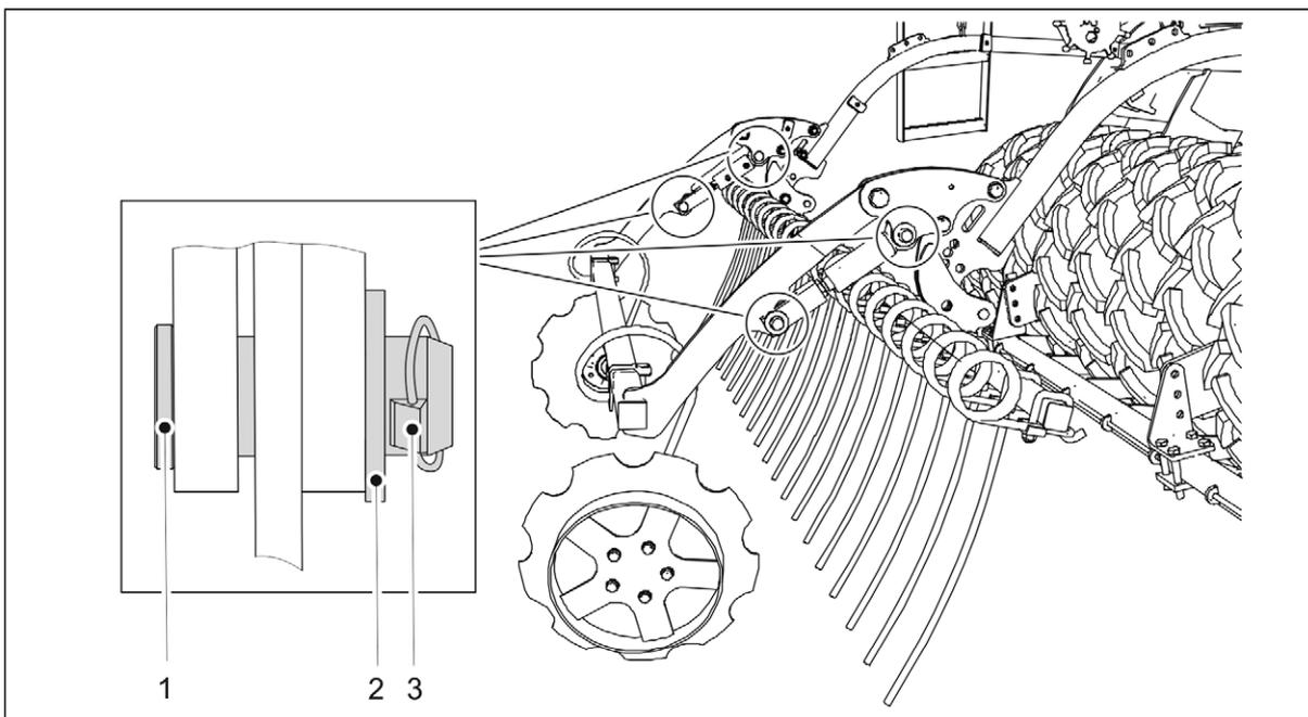
**Figure. 5.1.9. - 69. Mounting rear marker cylinders**
