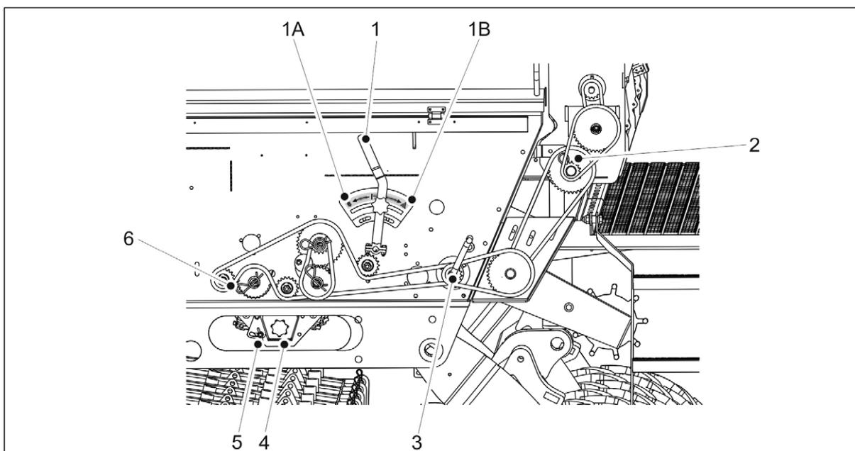
**Figure. 6.8.5. - 156. Seed calibration test on a machine without a gearbox.**
