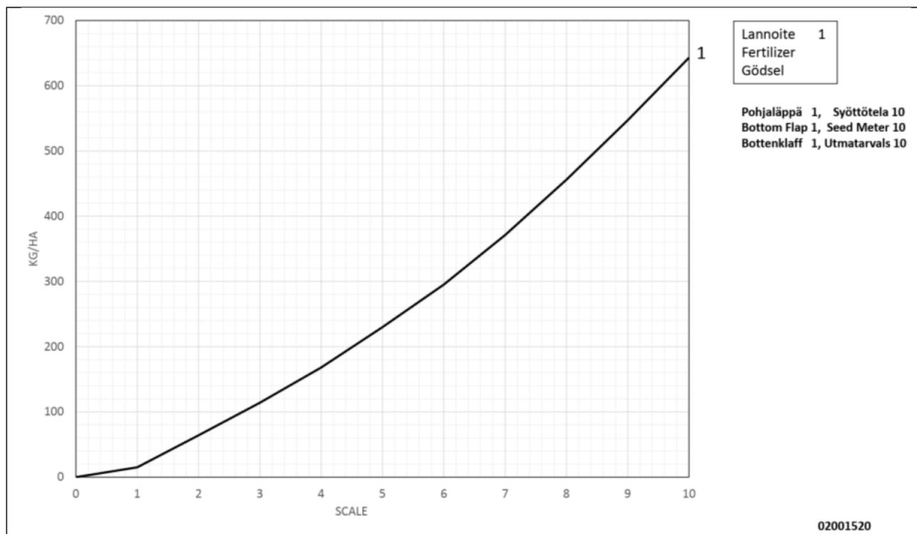
Figure. 6.5. - 118. Seeding table - seed and fertiliser gearbox 3
