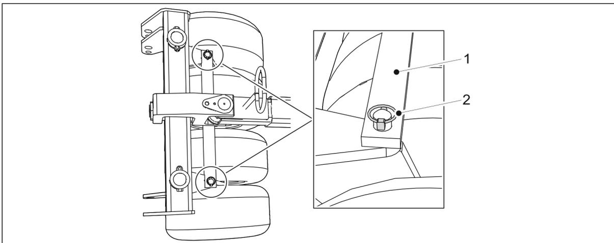
**Figure. 7.2.10. - 207. Detaching the wheel packer bar**
