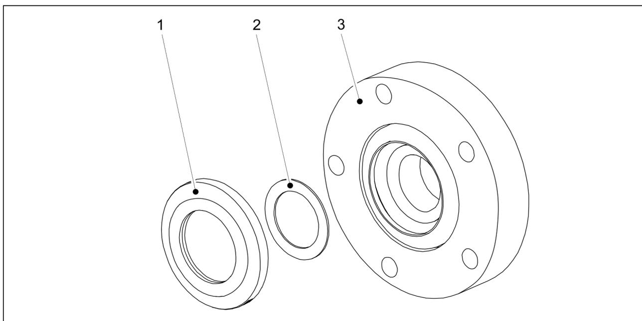
**Figure. 7.9.3.1. - 254. Bearing seal and shim**
