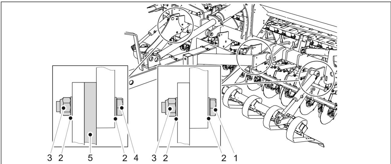
**Figure. 5.1.4. - 58. Mounting the front levelling board on a FX300**
