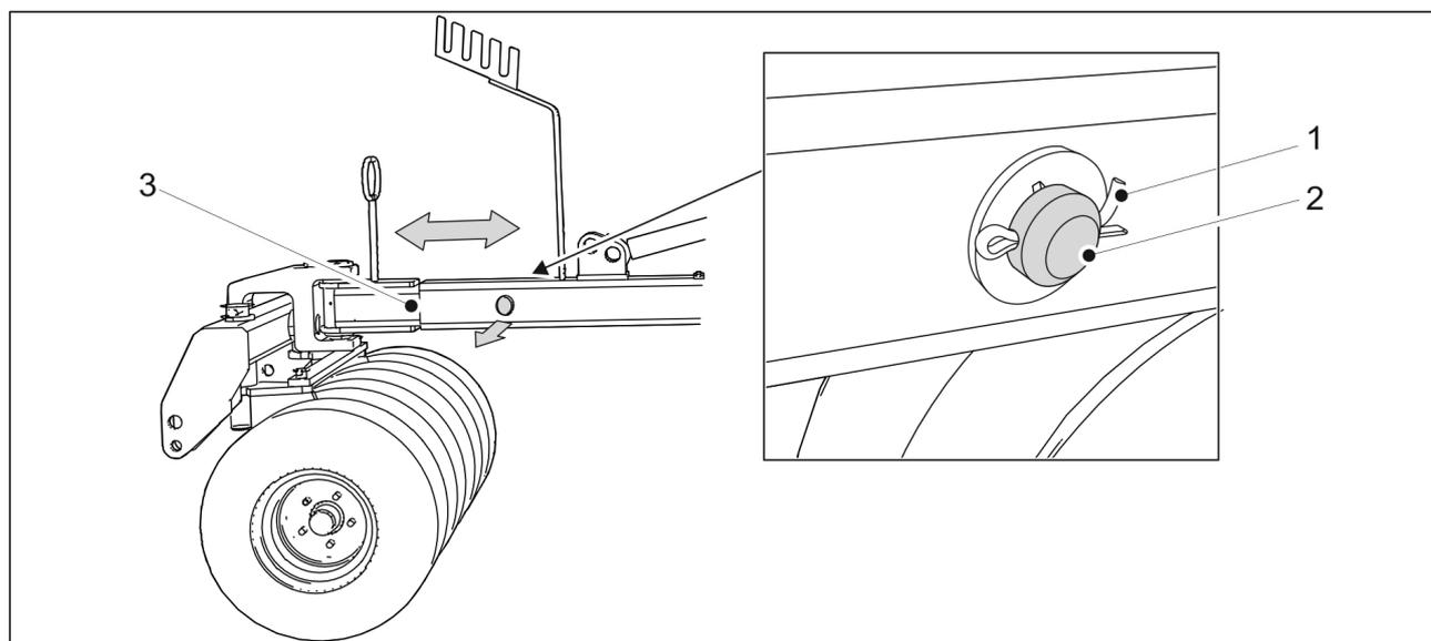
**Figure 5.3.1. - 83. Adjusting the length of the boom**
