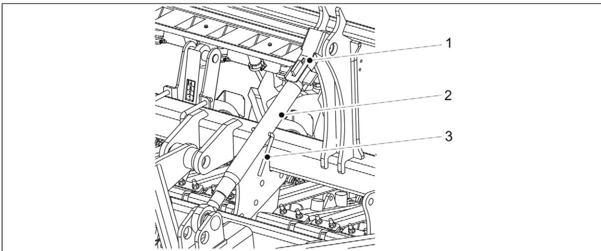
**Figure. 5.3.3. - 86. Adjustment with a turnbuckle**
