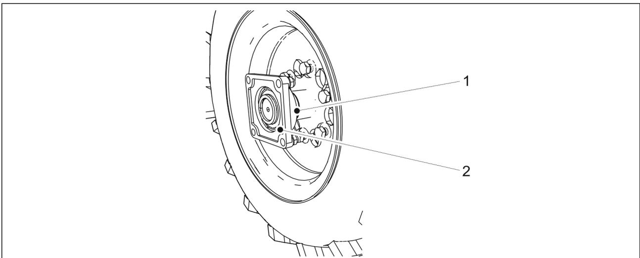
**Figure. 7.4.2. - 227. Detaching a flange bearing**
