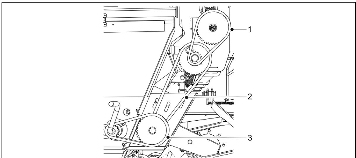
**Figure. 7.2.2.4. - 196. Lubricating the small seed hopper transmission chains**
