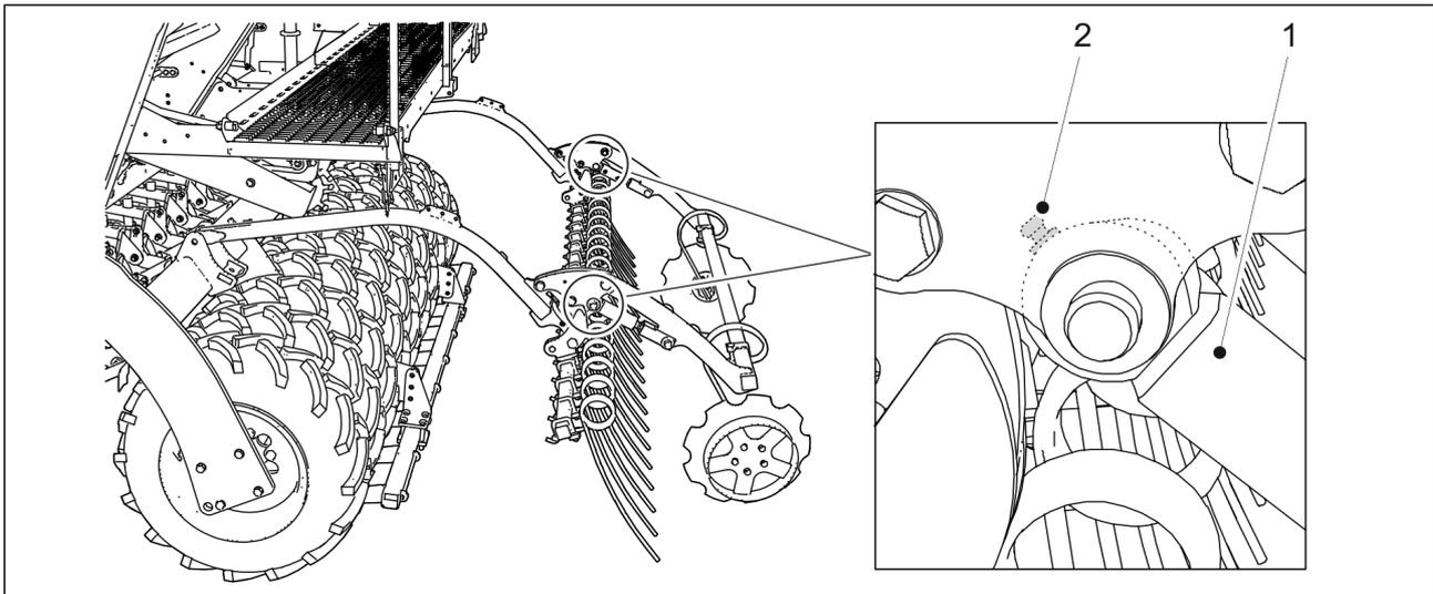
**Figure. 7.2.9. - 205. Rear marker cylinders**
