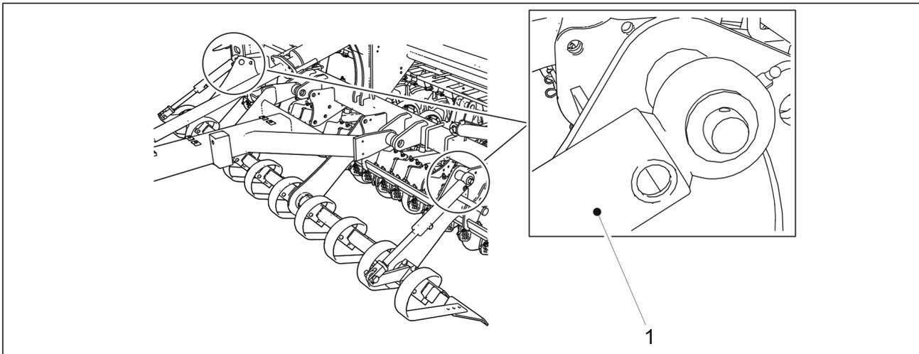
**Figure. 7.2.11. - 209. Front levelling board cylinders**
