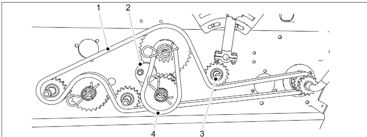
**Figure. 7.5.1. - 232. Tightening the chains in a machine without a gearbox**
