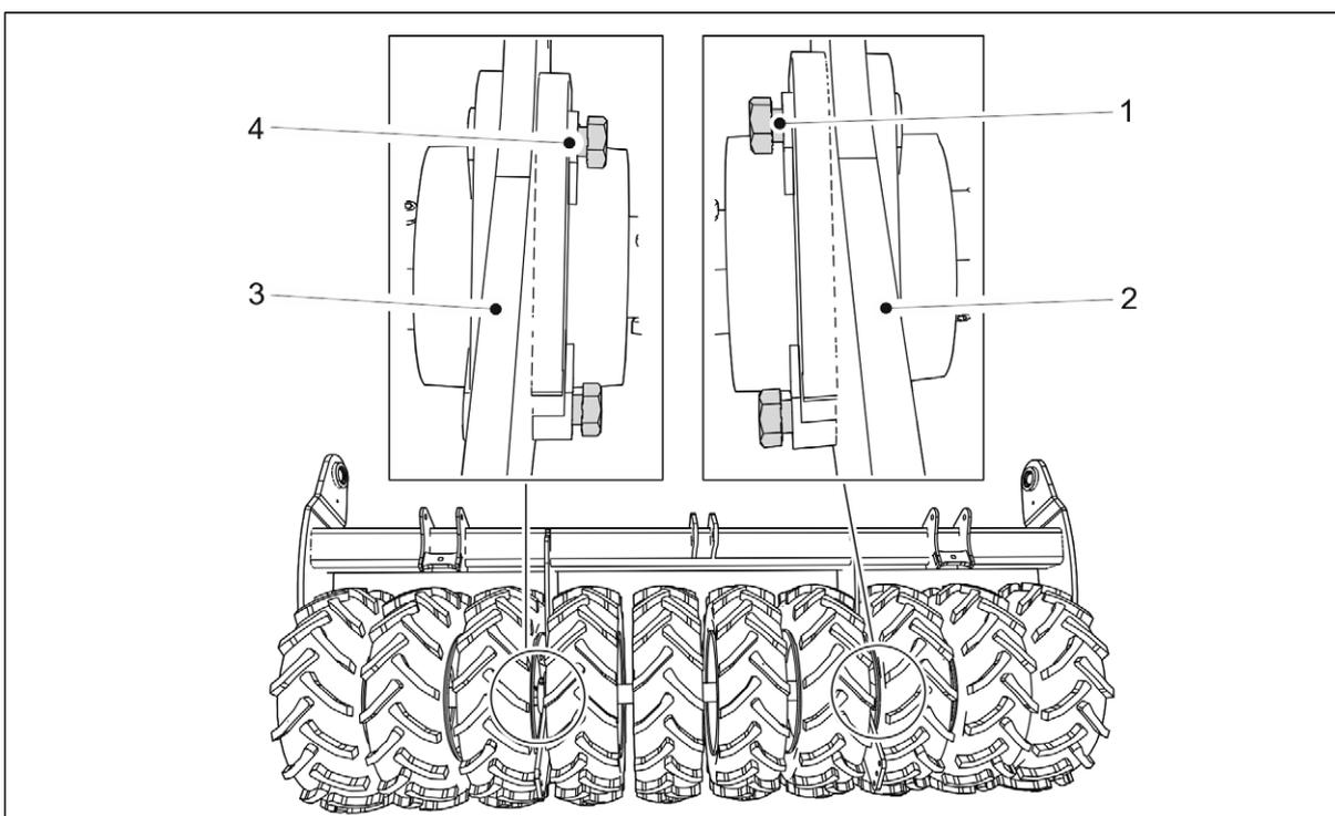
**Figure. 7.4.1. - 225. Turning the bolts**
