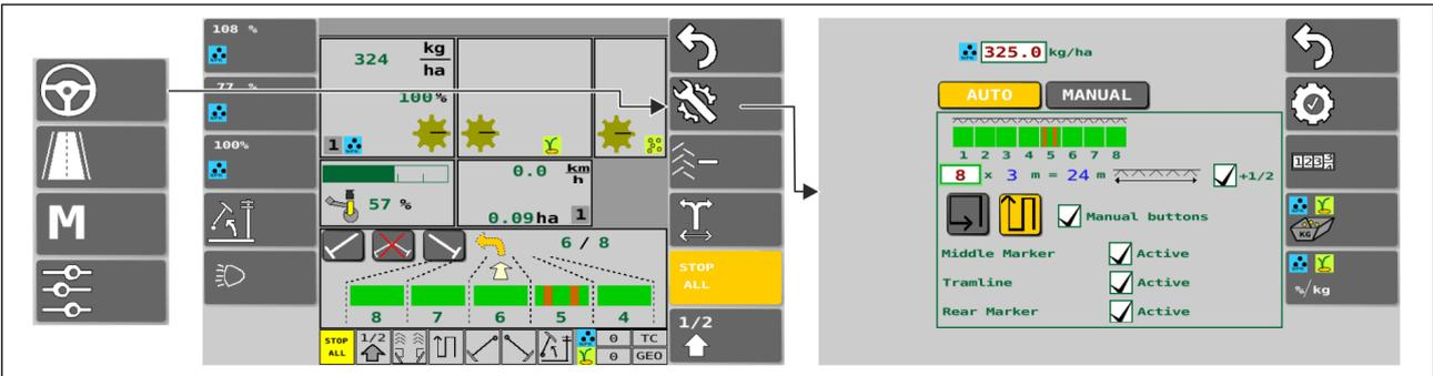
**Figure. 4.2.3. - 34. Drive screen and seeding settings (automatic)**
