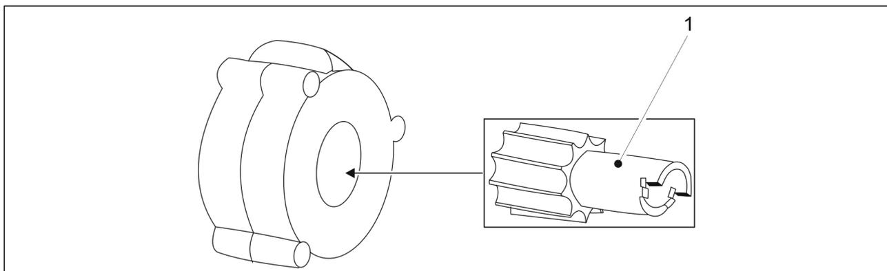
**Figure. 4.2.1.6. - 20. Notched feeder roller**
