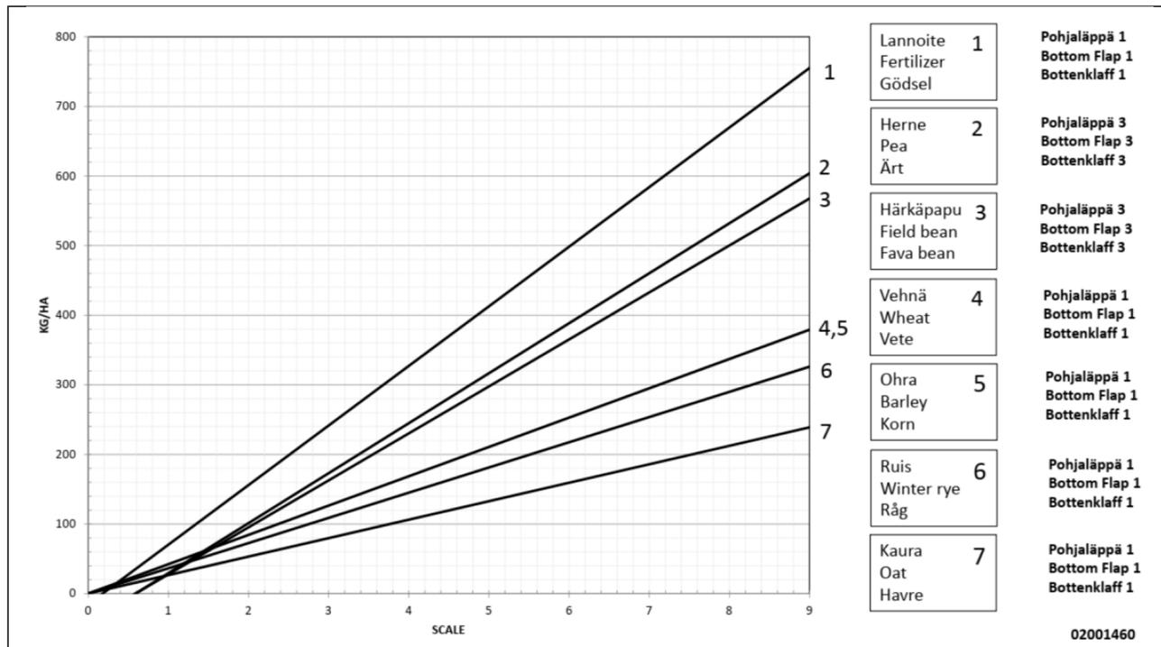
Figure. 6.5. - 111. Seeding table for machines with standard equipment
