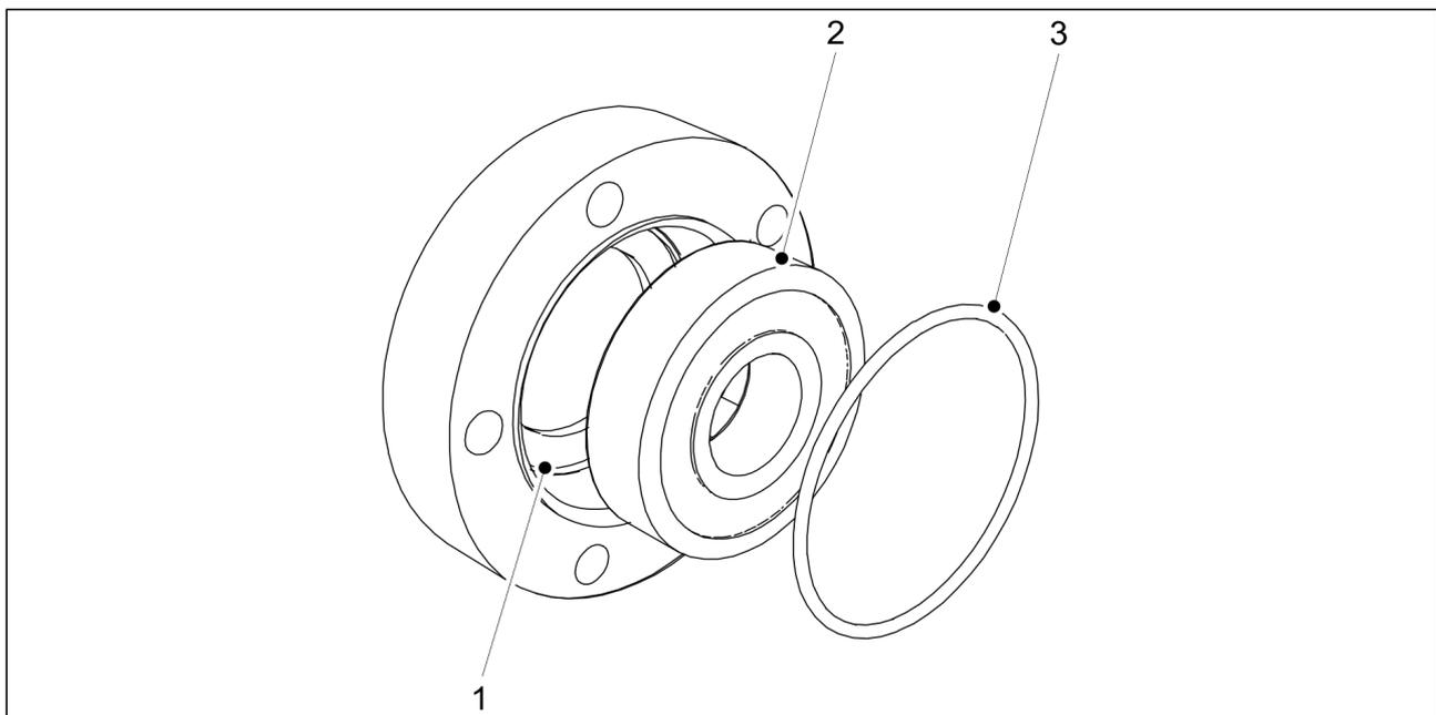
**Figure. 7.9.3.2. - 256. Installing the bearing**
