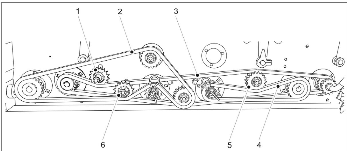
**Figure. 7.5.3. - 234. Tightening the chains in a machine with a dual gearbox**
