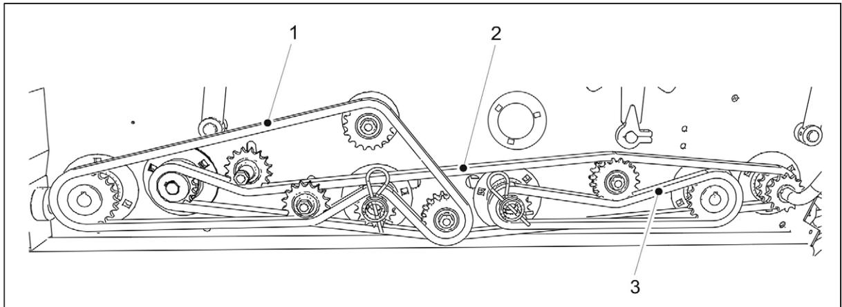
**Figure. 7.2.2.3. - 195. Lubricating chains in a machine with a dual gearbox**
