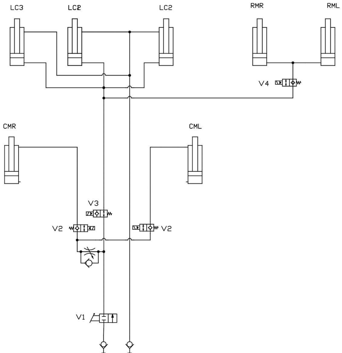
Lifting and lowering the machine (LC)
