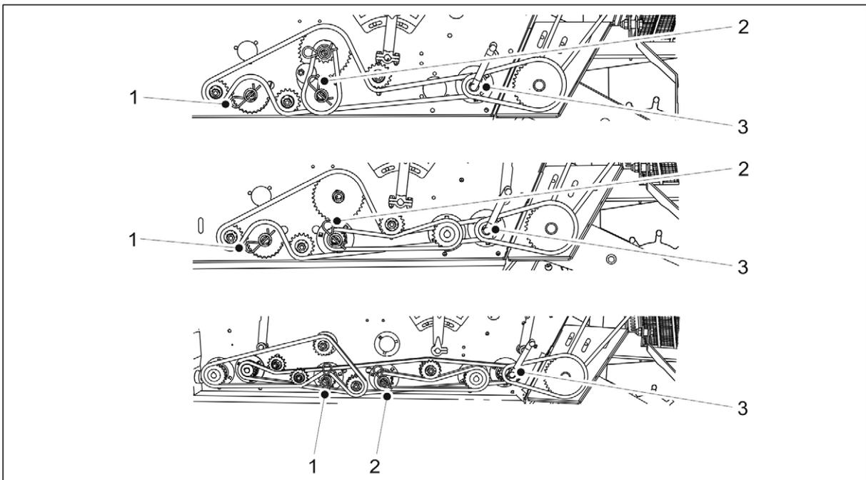
**Figure. 6.8.7. - 159. Calibration test of the small seed hopper. The top figure shows a machine without a gearbox; the middle figure shows a machine with a gearbox on the seed side; and the bottom figure shows a machine with a dual gearbox.**
