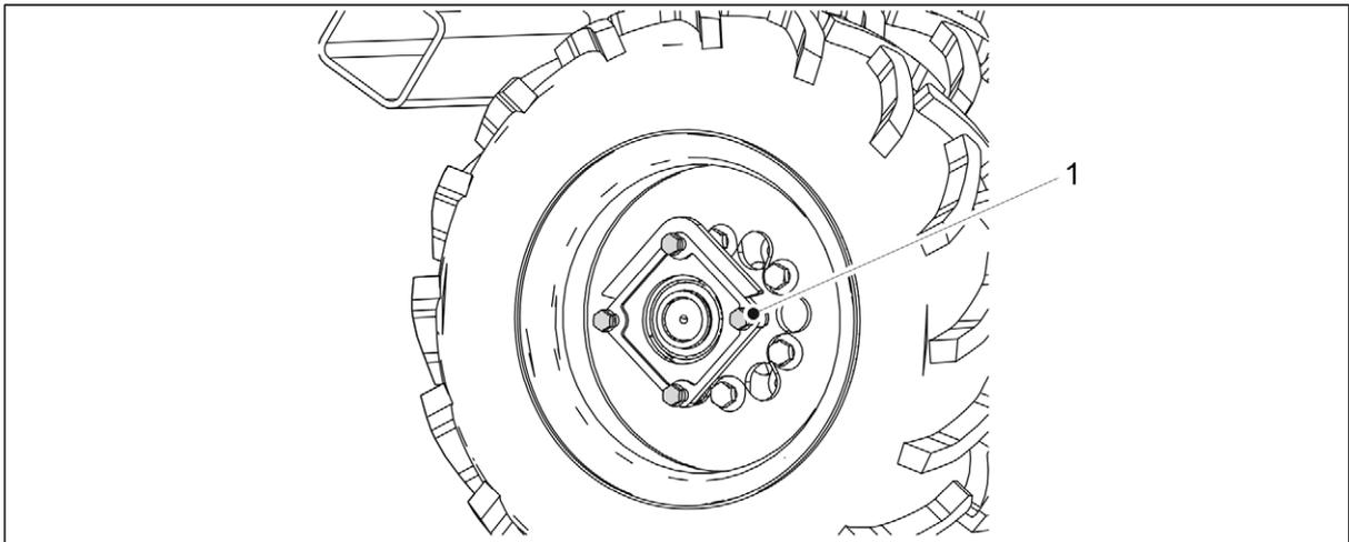
**Figure. 7.4.1. - 226. The wheel assembly is supported by bolts**
