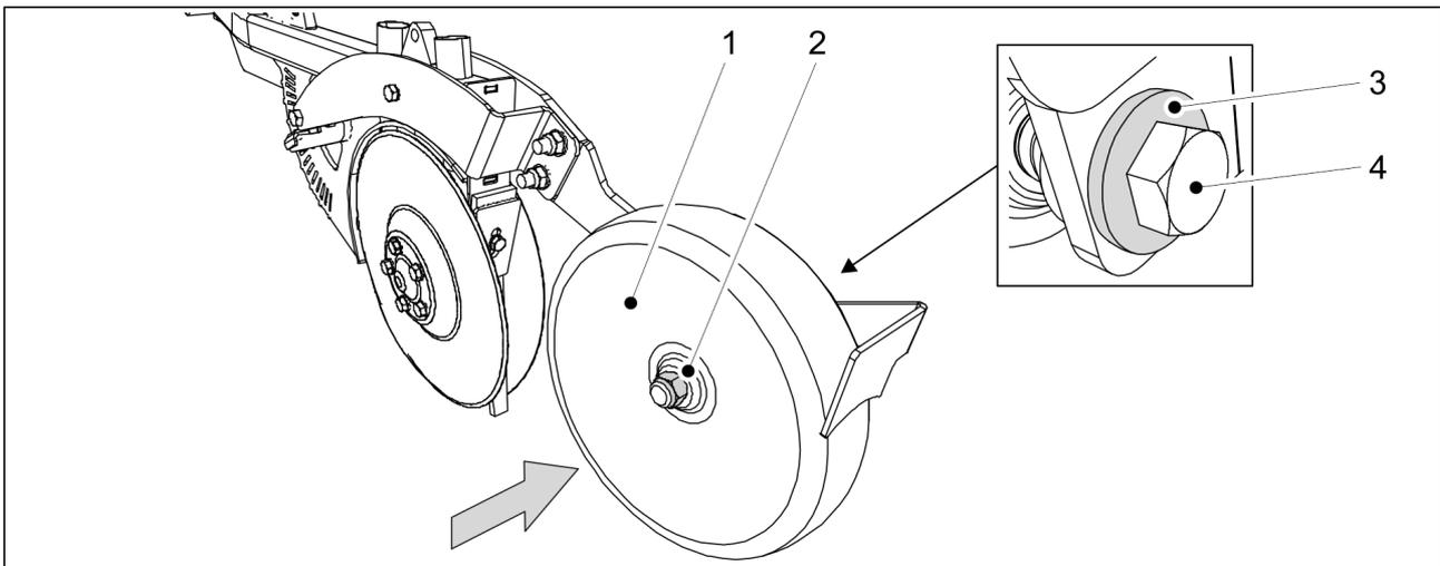
Figure. 7.9.4.2. - 259. Installing the covering wheel
