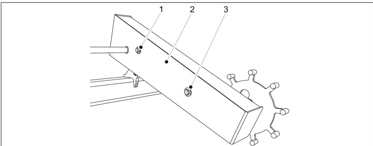
**Figure. 7.2.3.2. - 198. Cover of the wheel drive housing**
