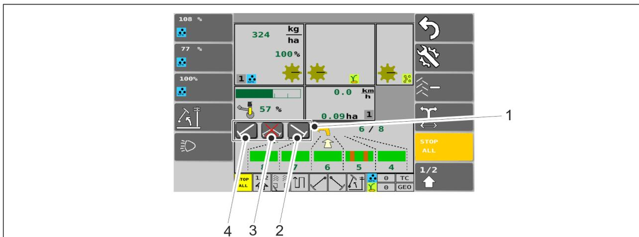
**Figure. 6.3.6. - 104. Middle markers manual control and forcing operation**
