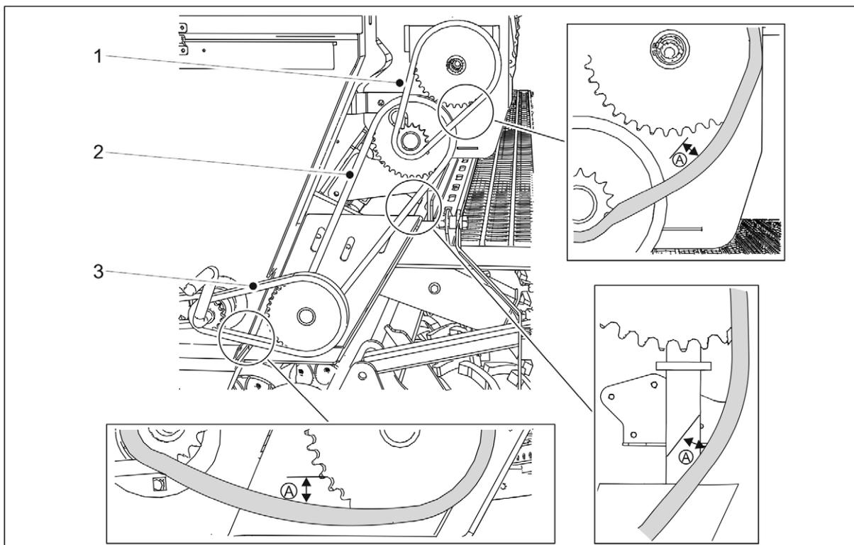
**Figure. 7.1.5.4. - 184. Checking the tightness of the chains in the small seed hopper transmission**
