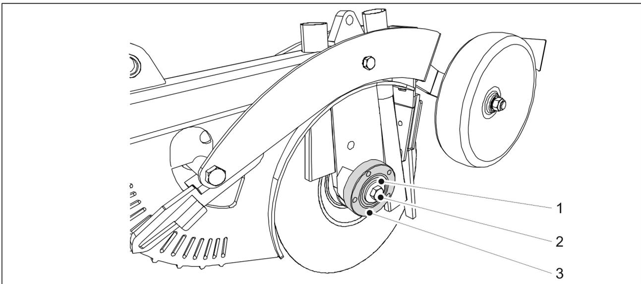
**Figure. 7.9.2.2. - 252. Installing the bearing housing**
