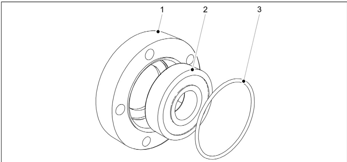
**Figure. 7.9.3.1. - 255. Removing the bearing and O-ring**
