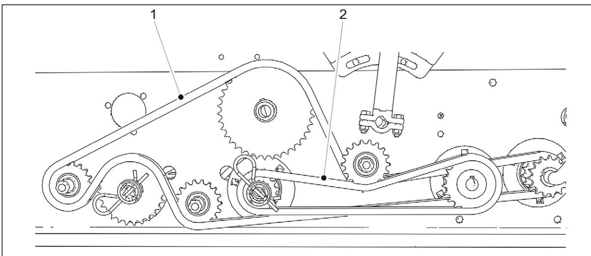
**Figure. 7.2.2.2. - 194. Lubricating the chains in a machine with a gearbox on the seed side**
