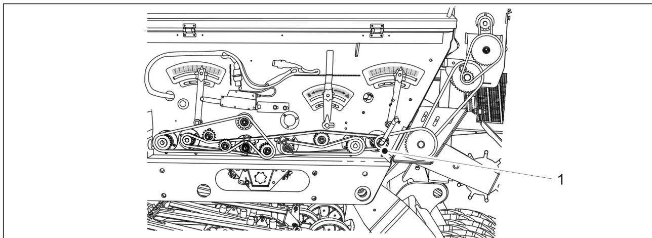
Figure. 6.8.4. - 151. Calibration test crank
