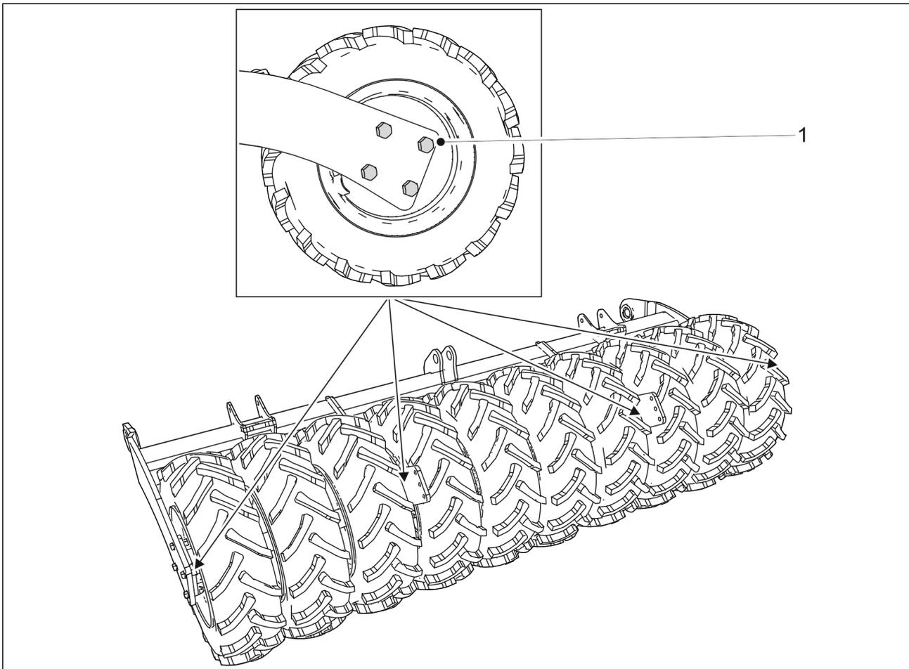
**Figure. 7.1.2.2. - 172. Flange bearing bolts of the transportation running gear**
