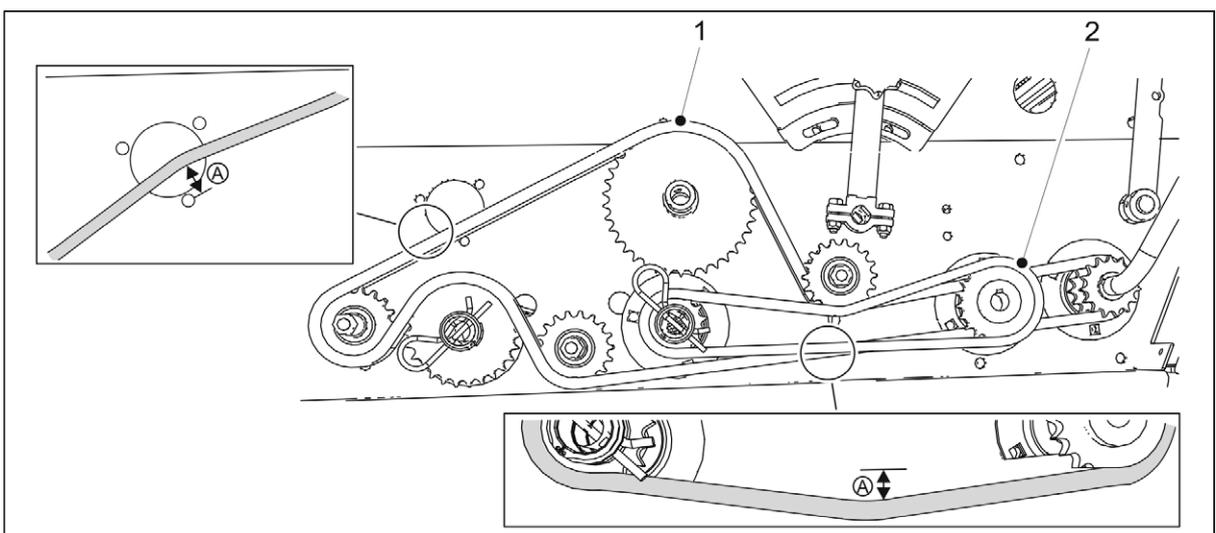
**Figure. 7.1.5.2. - 182. Checking the tightness of the transmission chains in a machine with a gearbox on the seed side**
