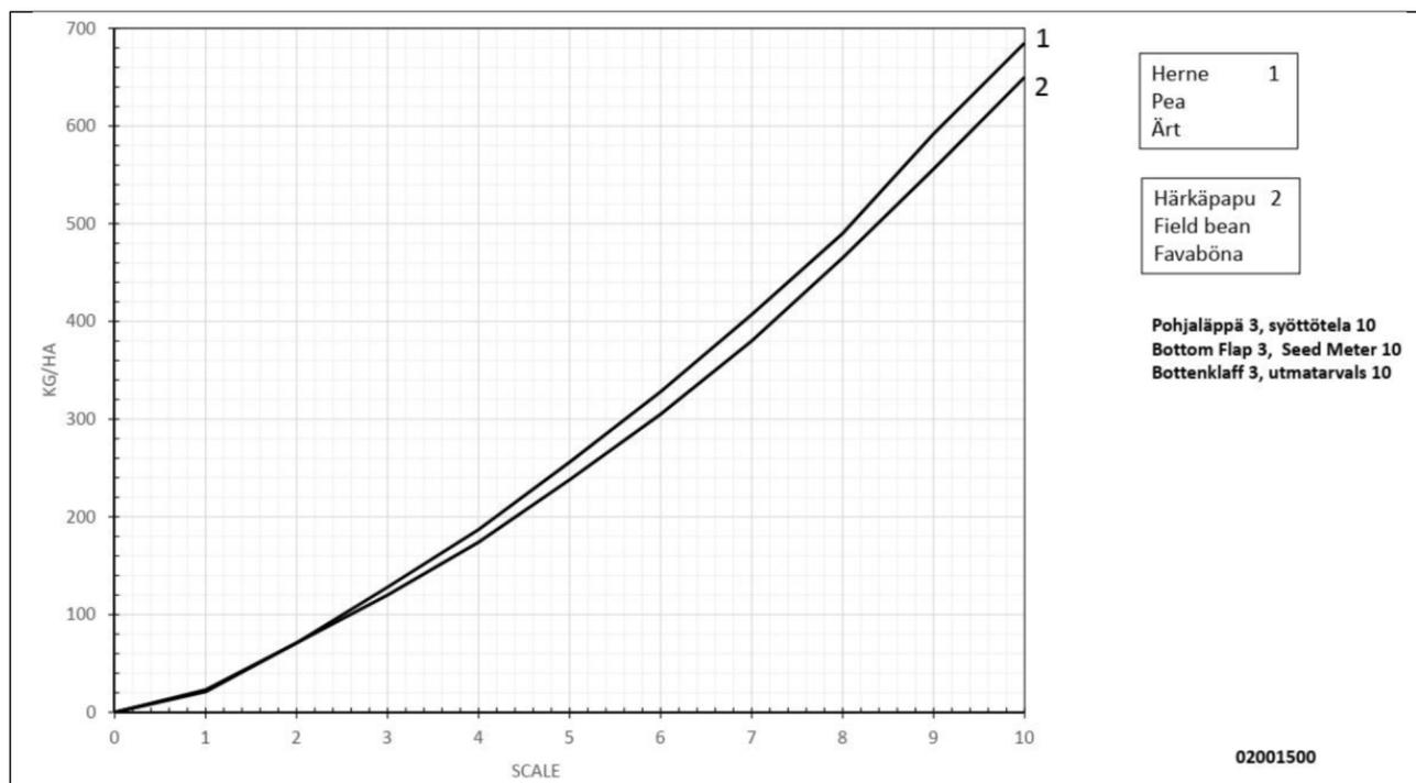
Figure. 6.5. - 117. Seeding table - seed and fertiliser gearbox 2
