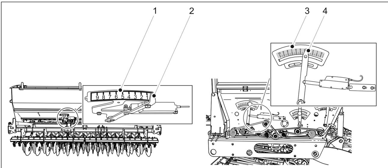
**Figure. 7.1.14. - 192. Checking the functioning of the adjusting of fertiliser target rate** On the left, a machine without a gearbox and, on the right, a machine equipped with a gearbox on the seed side (basic model). On the right, a machine with a dual gearbox (machine with gearbox).
