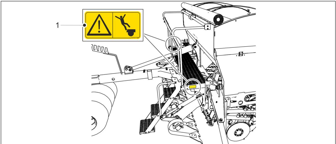
**Figure. 3.3. - 9. Labels on the front platform**
