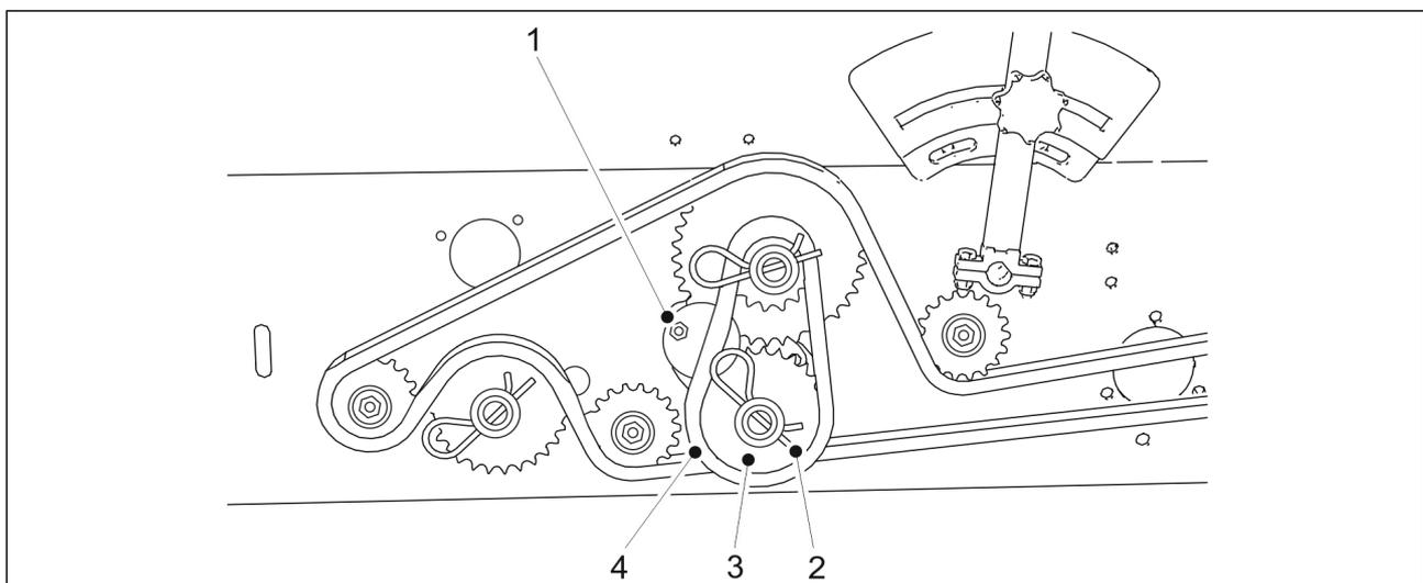
**Figure. 6.6.6. - 122. Changing the chain gears and chain**
