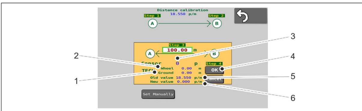
**Figure. 7.10.2.2. - 268. Manual calibration of travel distance 3**
