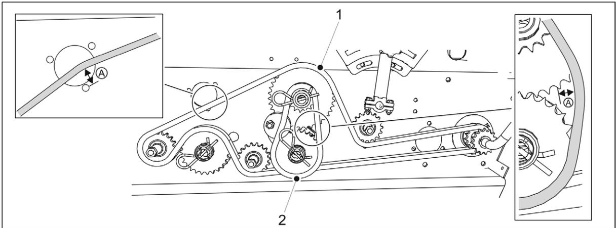
**Figure. 7.1.5.1. - 181. Checking the tightness of chains in a machine without a gearbox**
