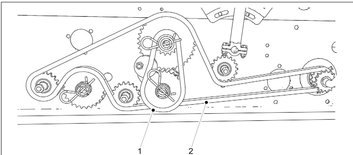
**Figure. 7.2.2.1. - 193. Lubricating the chains in a machine without a gearbox**
