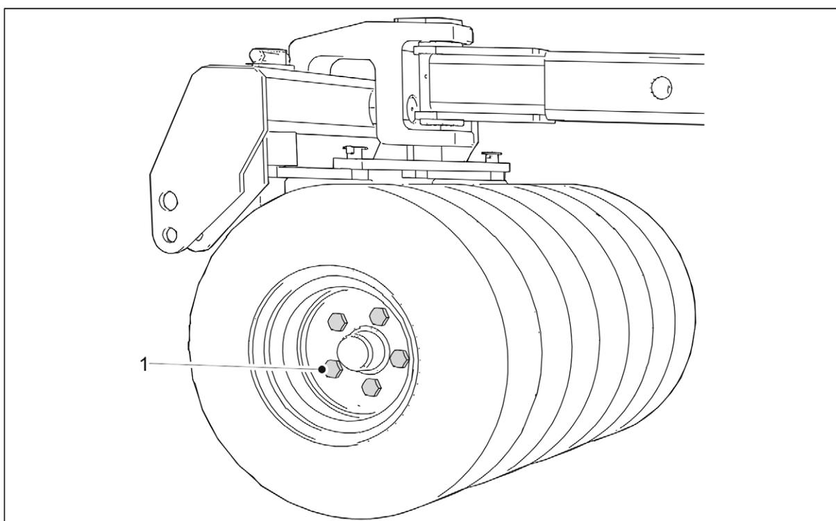
**Figure. 7.1.2.3. - 174. Wheel bolts of the wheel packer**
