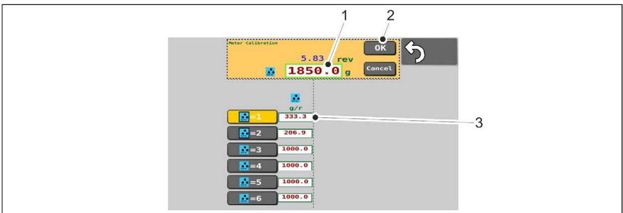
**Figure. 6.8.4. - 154. Entering the weighing result**
