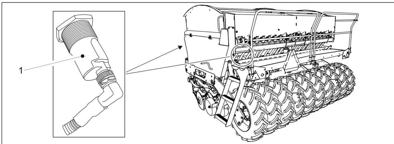
**Figure. 4.2.1.5. - 18. Hopper level sensors**
