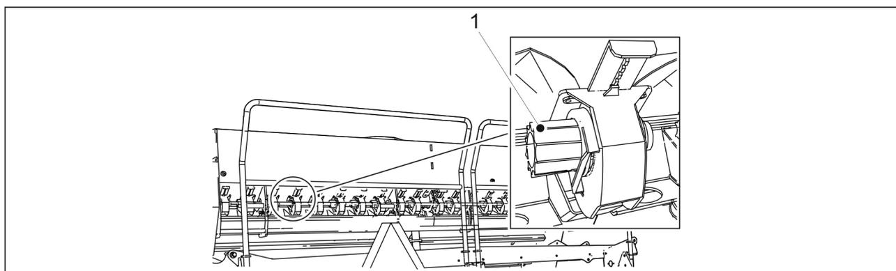
**Figure. 7.3.6. - 218. Feeder roller**
