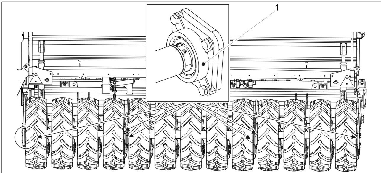
Figure. 7.2.5. - 201. Wheel axle bearings
