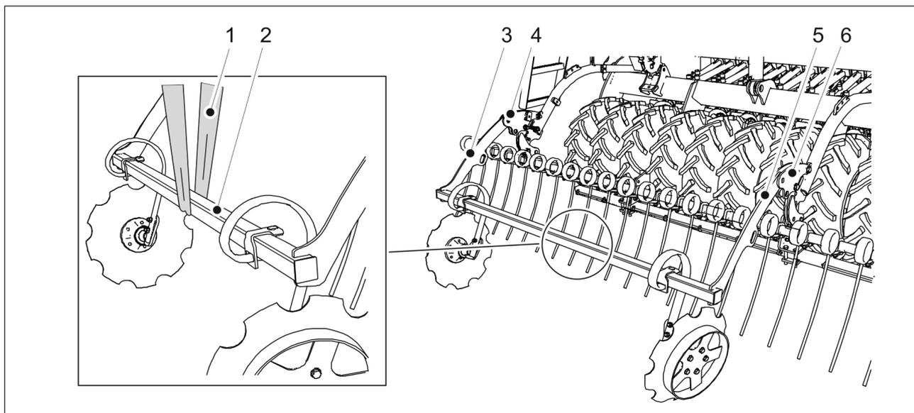
**Figure. 5.1.9. - 67. Lifting the rear markers**
