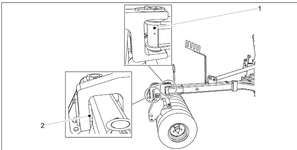
**Figure. 6.1. - 92. Wheel packer pins**
