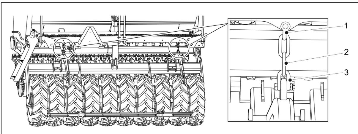
**Figure. 5.1.8. - 64. Attaching the rear harrow chains**
