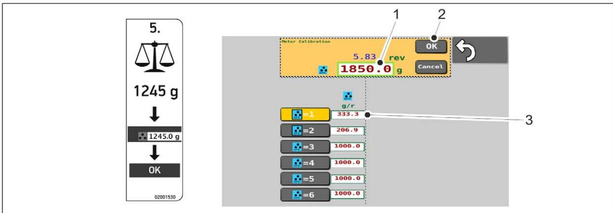
**Figure 6.8.3. - 145. Entering the weighing result**
