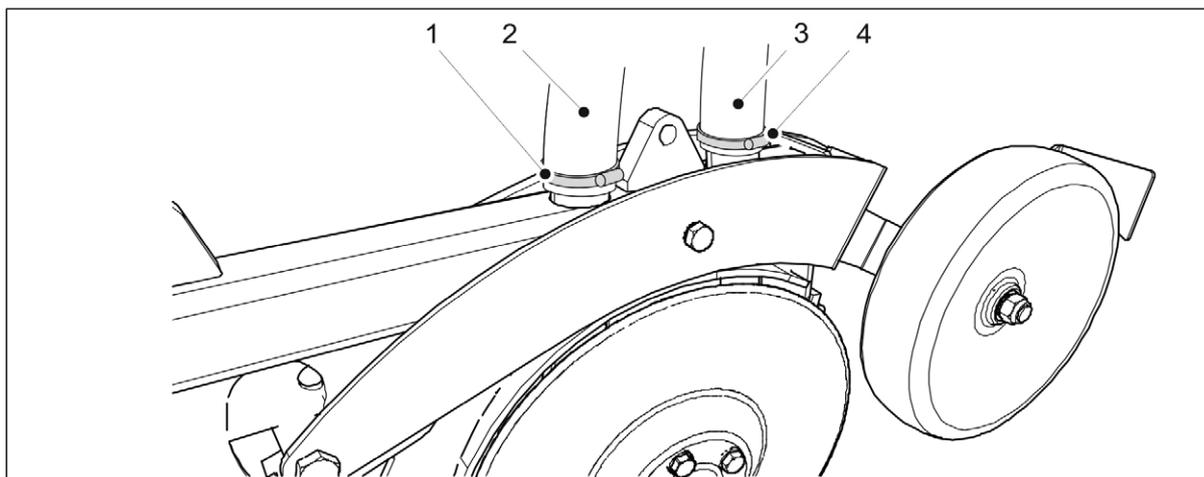
**Figure. 7.9.1.2. - 249. Connecting coultter hoses**
