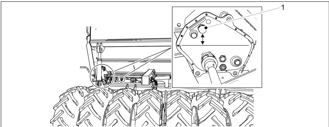
**Figure. 7.1.12. - 190. Gearbox oil level**
