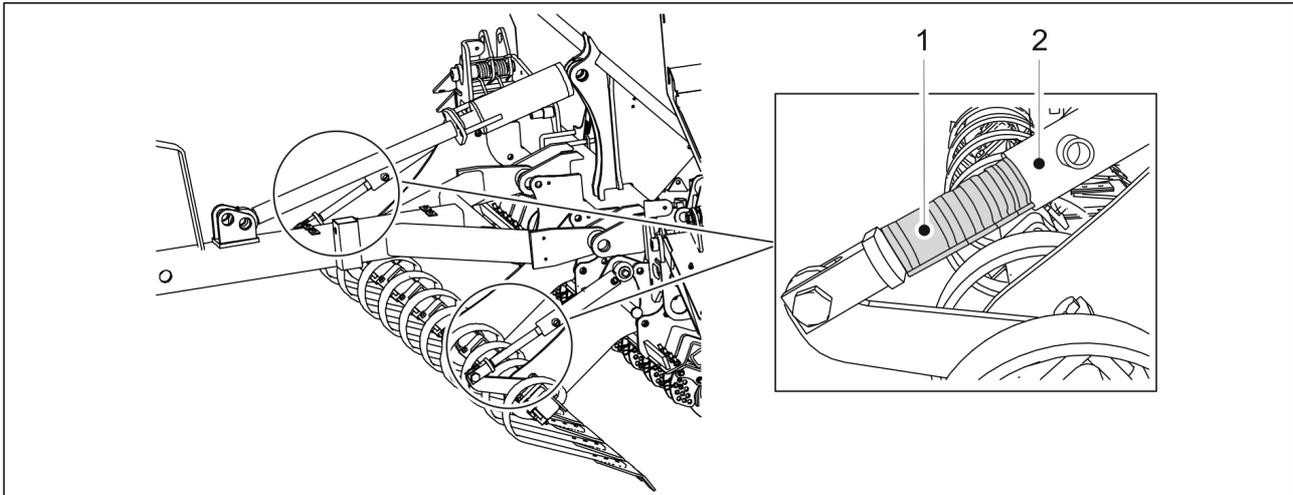
**Figure. 6.12. - 164. Adjusting the front levelling board**
