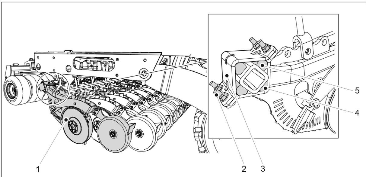
**Figure. 7.9.1.2. - 247. Fastening the coulter**
