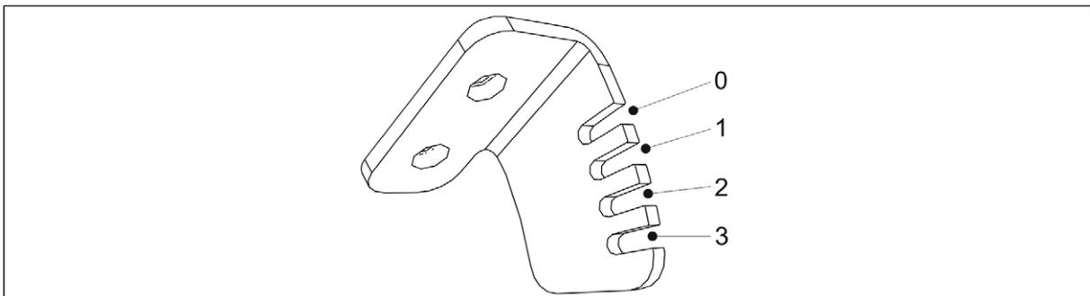
**Figure. 6.6.11. - 130. Bottom flap positions in the feeder units of the small seed hopper**
