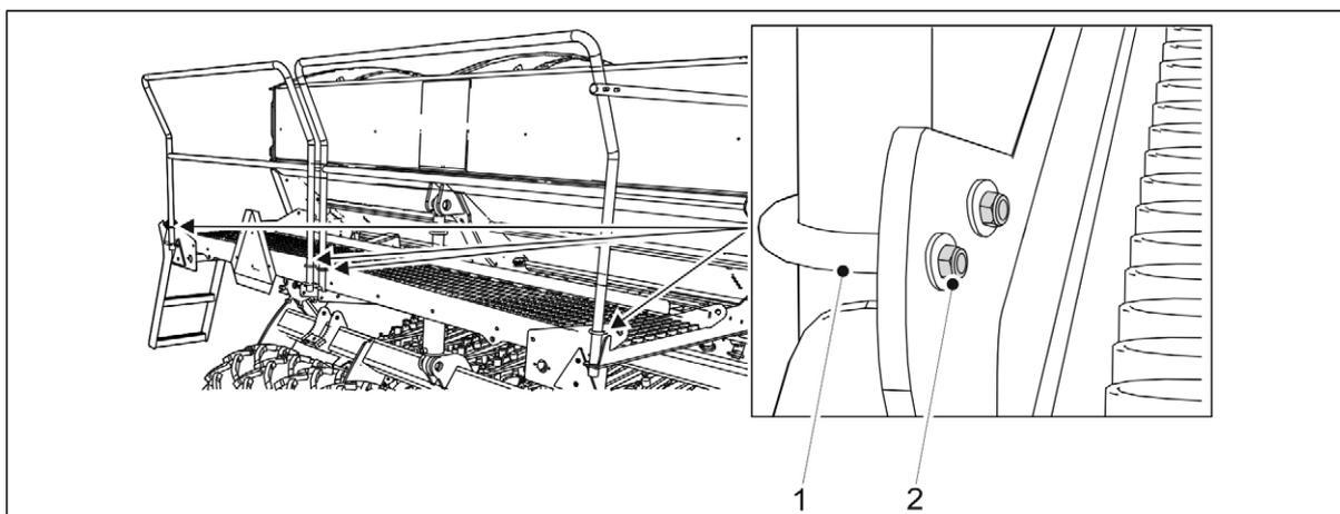
**Figure. 7.1.2.5. - 178. Working platform U-bolts**
