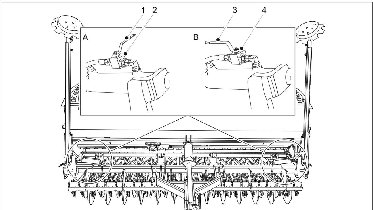
**Figure. 3.4. - 10. Middle marker ball valves**
