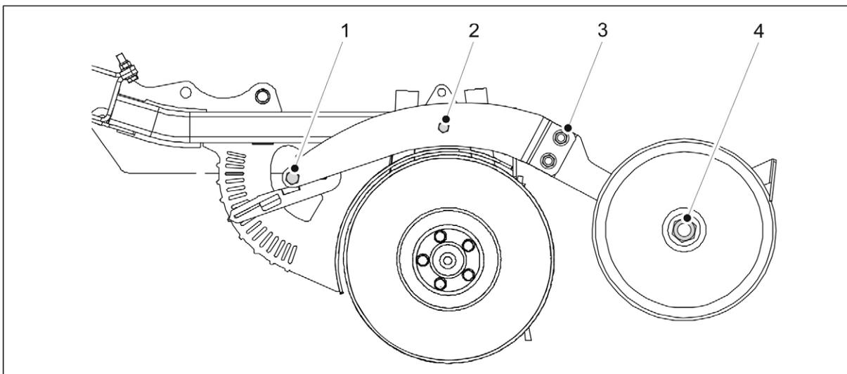
**Figure. 7.1.2.4. - 176. Bolts of the coulters covering wheel and depth adjustment**
