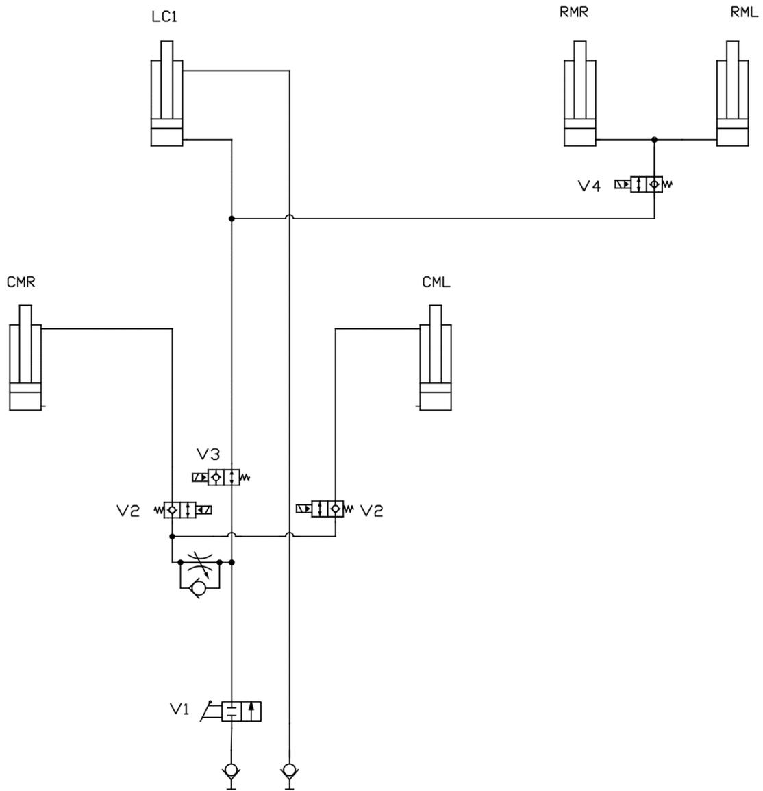
Lifting and lowering the machine (LC)
