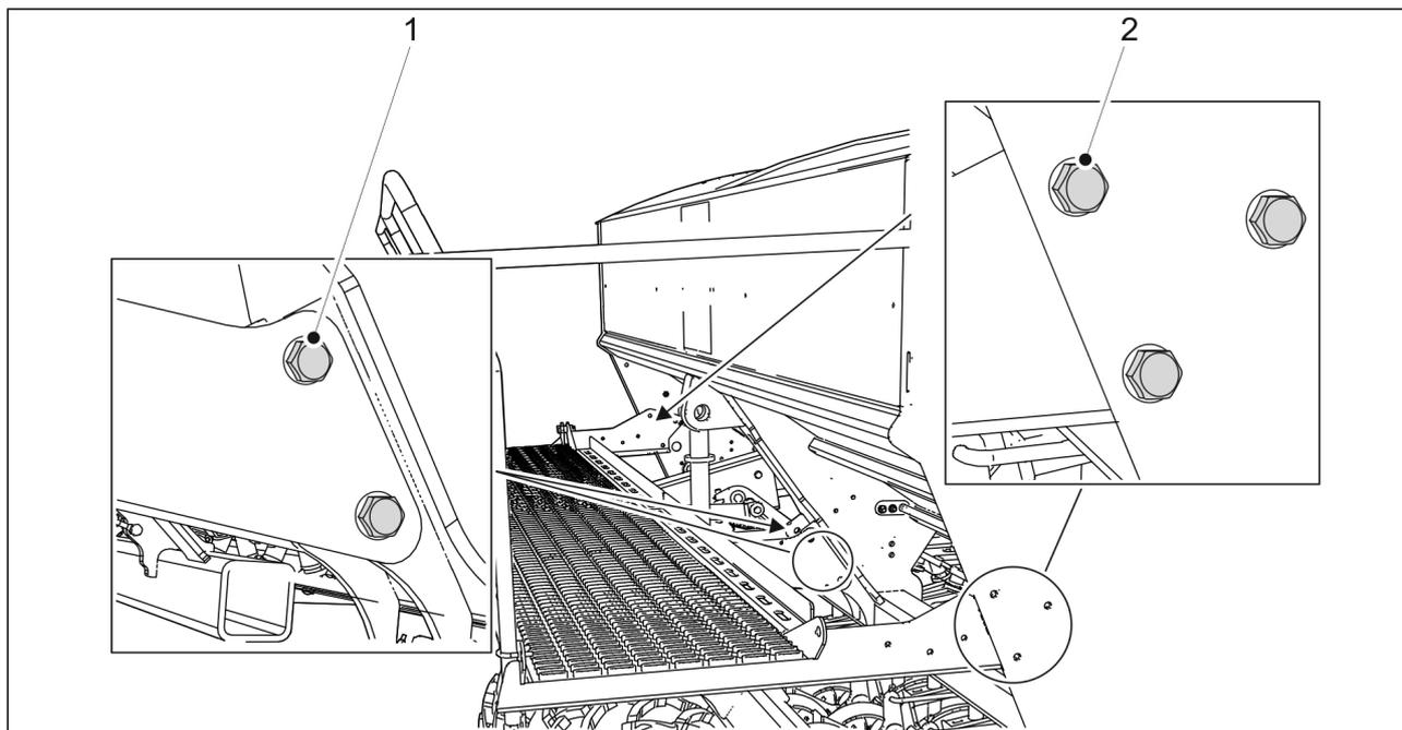
**Figure. 7.1.2.5. - 177. Working platform bolts**
