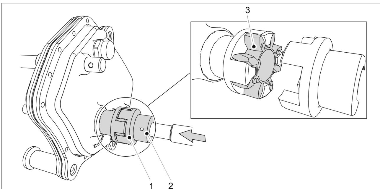
**Figure. 7.7.2.2. - 241. Installing the clutch**
