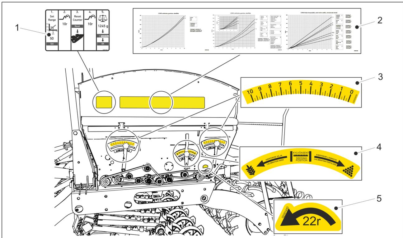
**Figure. 3.3. - 5. Seeding and adjustment labels on the left side of the seed drill**
