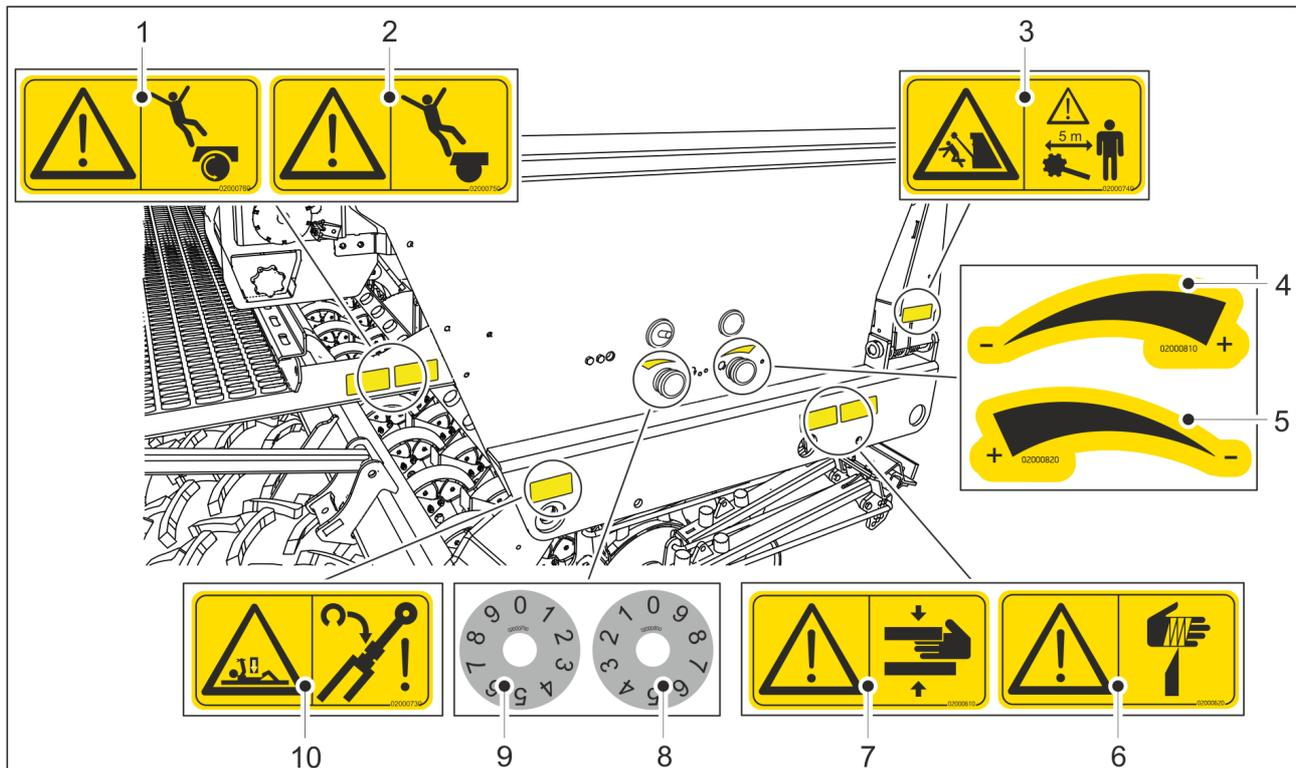
**Figure 3.3. - 3. Right side labels of the seed drill**
