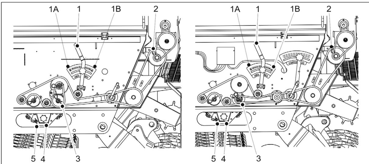
**Figure. 6.8.3. - 137. Calibration test with adjusting of fertiliser target rate** On the left, a machine without a gearbox and on the right, a machine equipped with a gearbox on the seed side.
