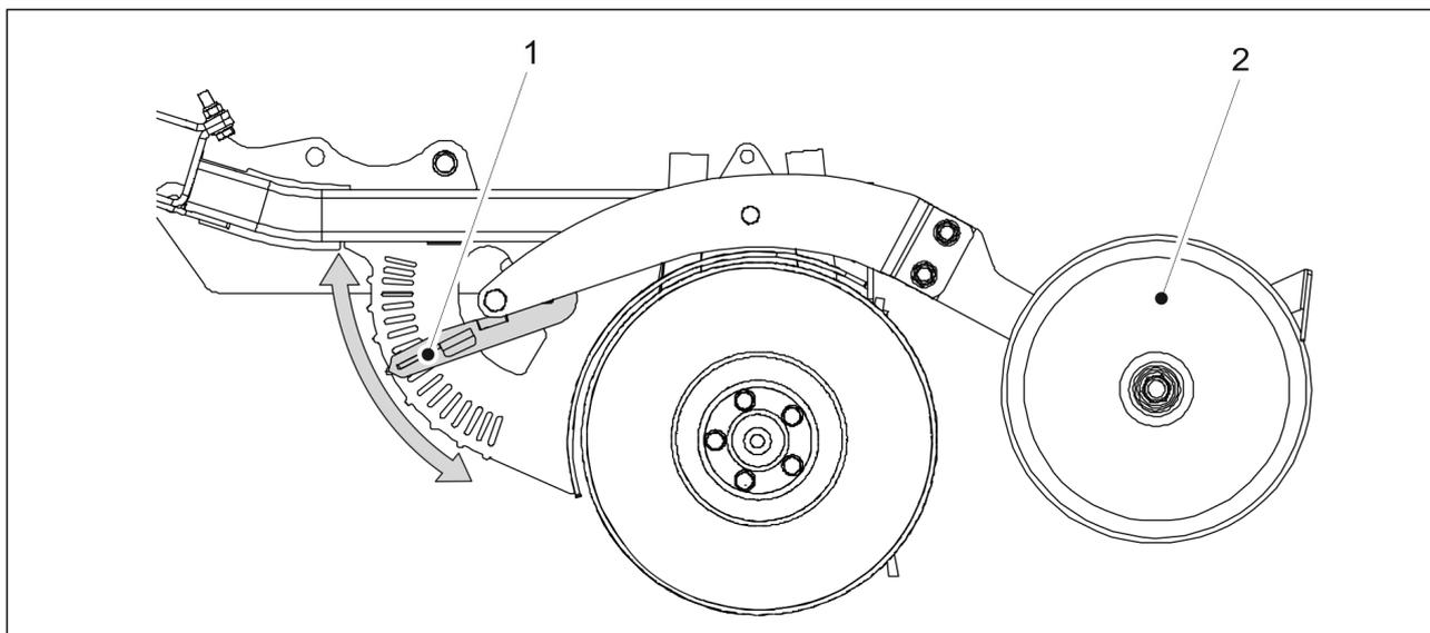
**Figure 6.9. - 160. Adjusting the seeding depth of the coulter**
