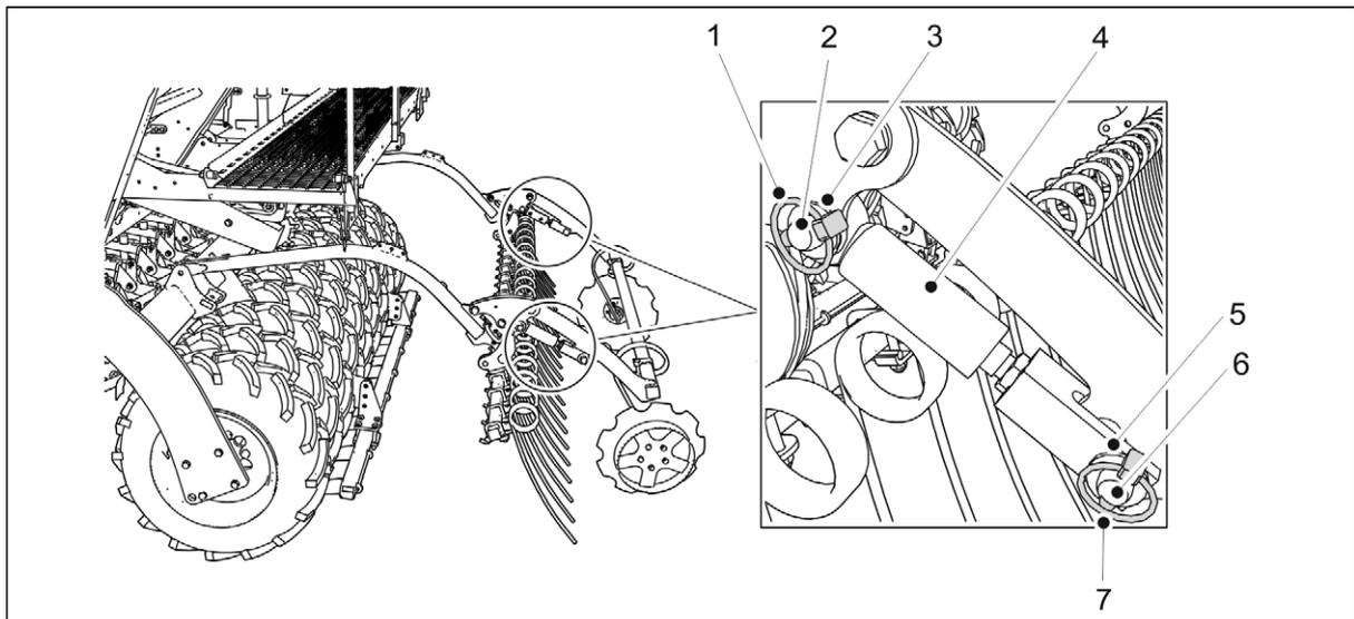
**Figure. 7.4.1. - 220. Removal of the rear marker cylinders.**
