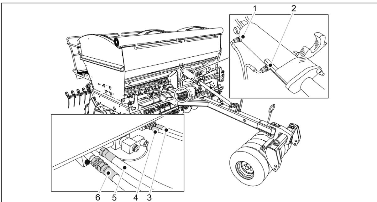
**Figure. 5.1.1. - 54. Connecting the hydraulic hoses**
