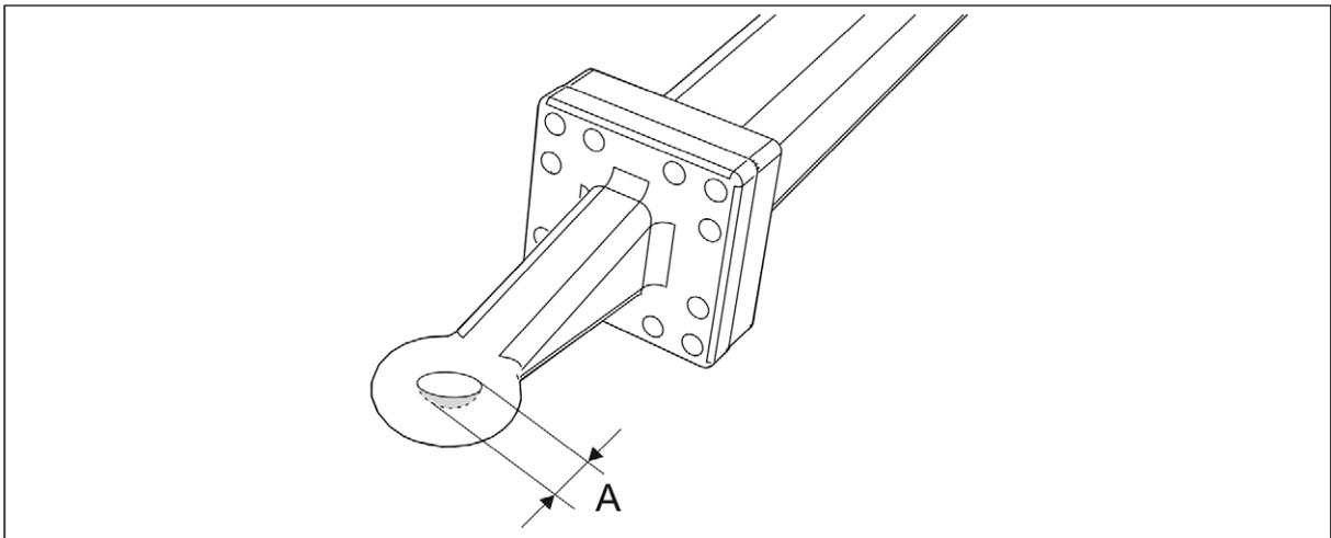
**Figure. 7.1.11. - 189. Wear in the towing eye**
