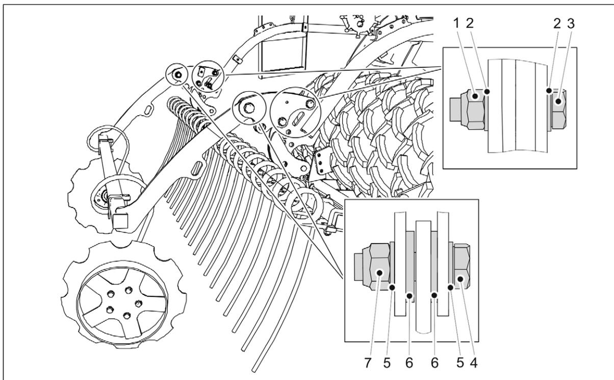
**Figure. 5.1.9. - 68. Mounting rear markers to the rear harrow**
