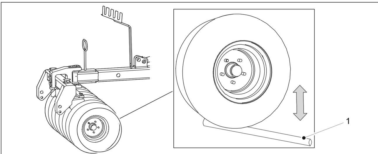
Figure. 7.1.4. - 180. Checking the bearing clearance of the wheel packer hubs
