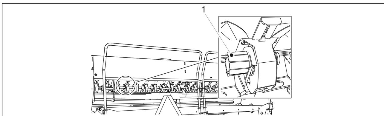
**Figure. 6.6.10. - 128. Feeder roller of the small seed hopper**
