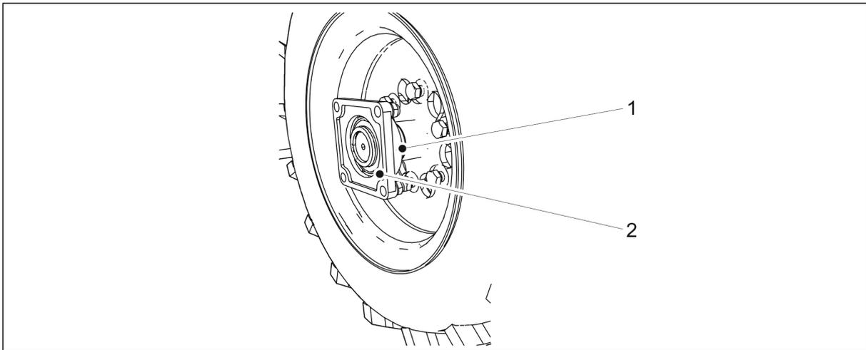
**Figure. 7.4.3. - 230. Fastening the bearing**
