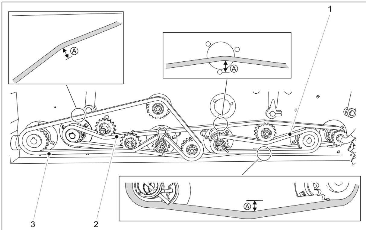
**Figure. 7.1.5.3. - 183. Checking the tightness of the transmission chains in a machine with a dual gearbox**
