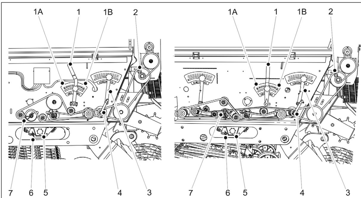
**Figure. 6.8.6. - 157. Seed calibration test. On the left, a machine with a gearbox on the seed side and on the right, a machine equipped with a dual gearbox.**
