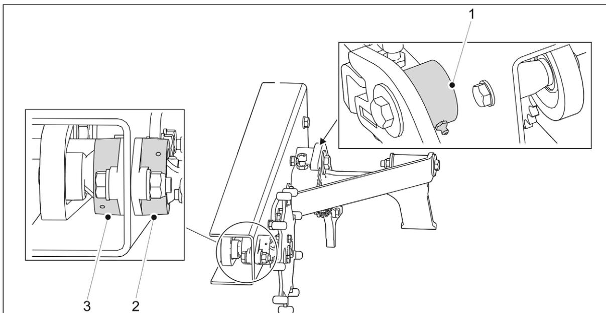
**Figure. 7.2.3.2. - 199. Lubricating wheel axle bearings**
