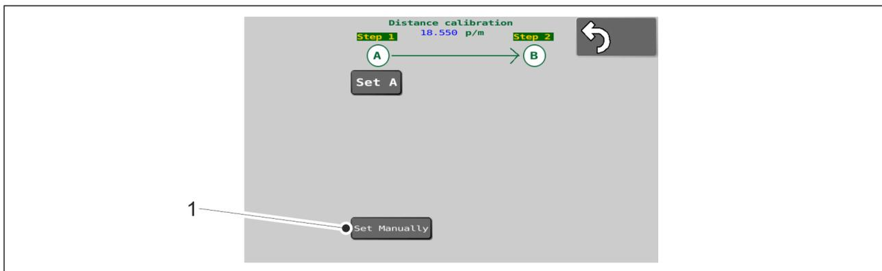
**Figure. 7.10.2.2. - 266. Manual calibration of travel distance 1**
