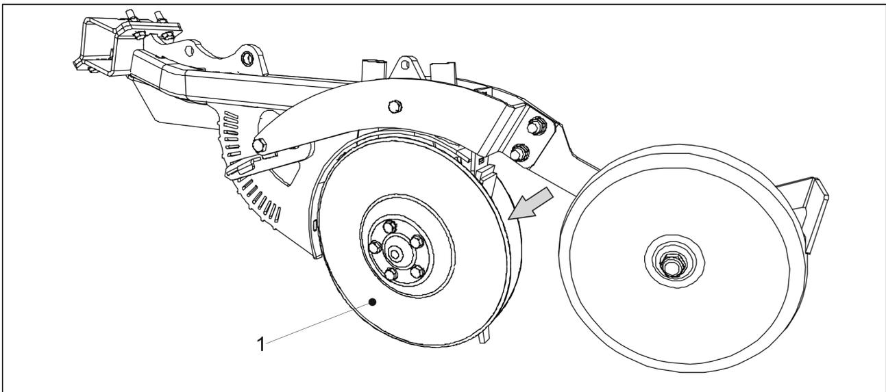
**Figure. 7.3.4. - 216. Discs of the coulters**
