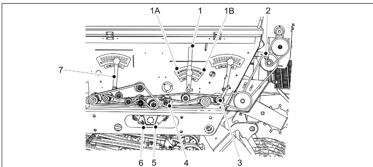
**Figure. 6.8.2. - 136. Fertiliser calibration test on a machine with a dual gearbox**
