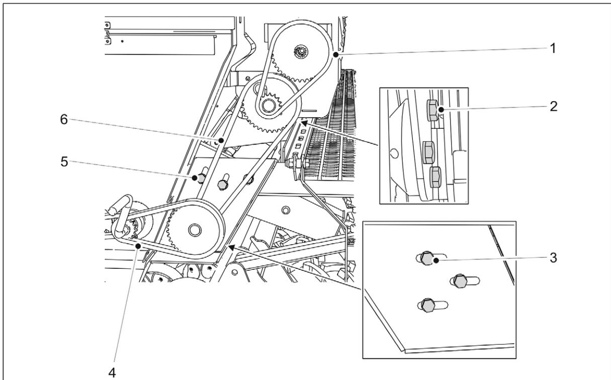
**Figure. 7.5.4. - 235. Tightening the transmission chains of the small seed hopper**
