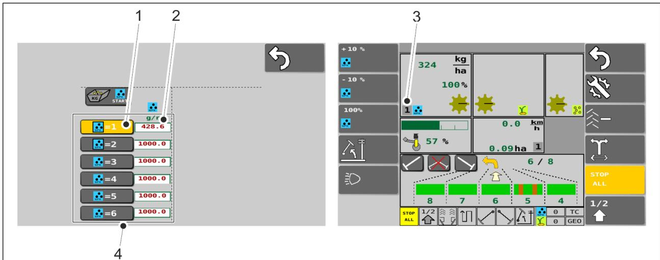
Figure. 6.3.2. - 95. Calibration test result memory slots
