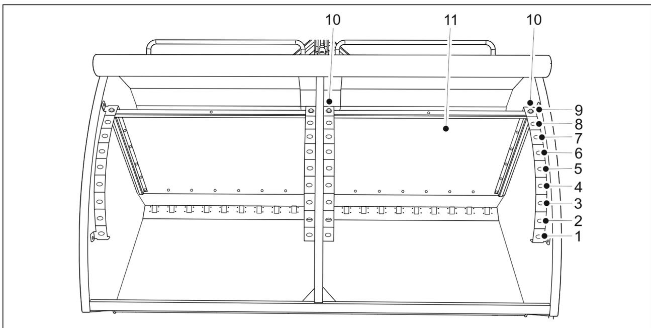
**Figure. 6.6.4. - 119. Adjusting the hopper divider**
