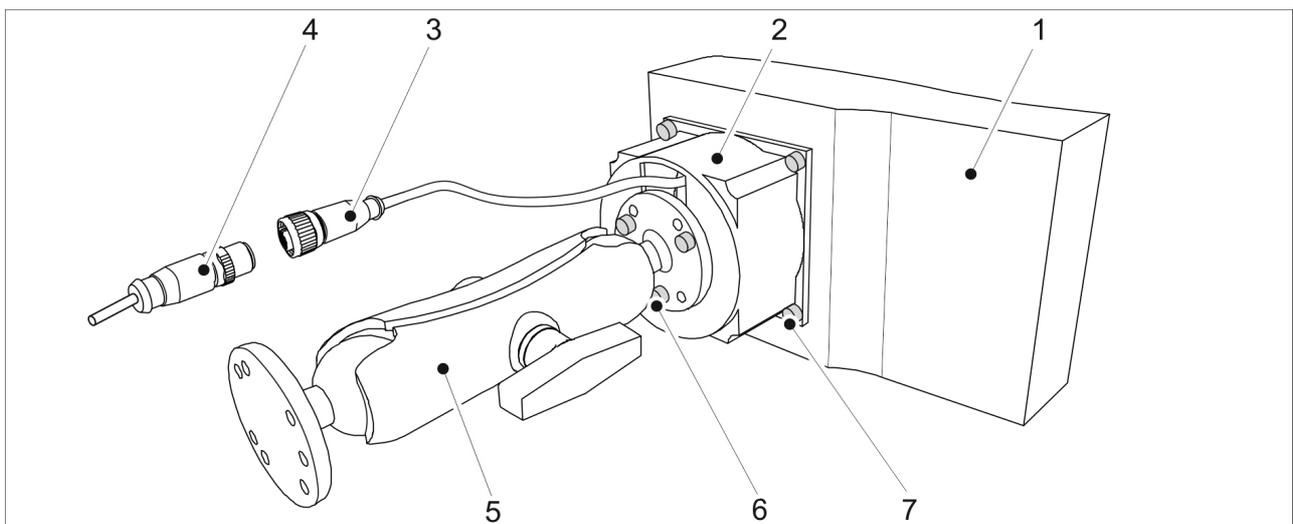
**Figure. 5.2.2. - 74. Installing the SeedPilot control panel**
