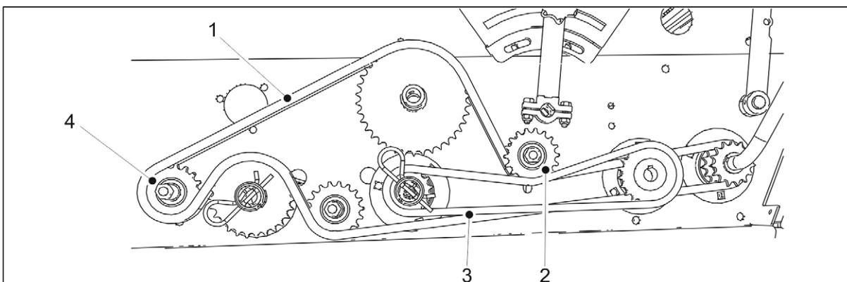
**Figure. 7.5.2. - 233. Tightening the chains in a machine with a gearbox on the seed side**
