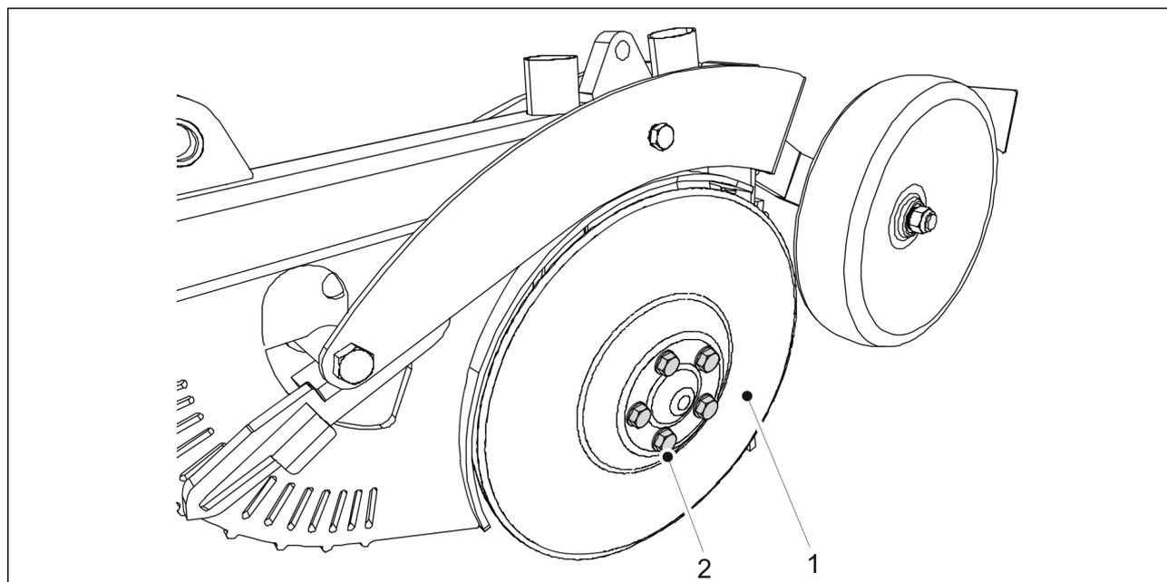
**Figure. 7.9.2.1. - 250. Detaching a disc**
