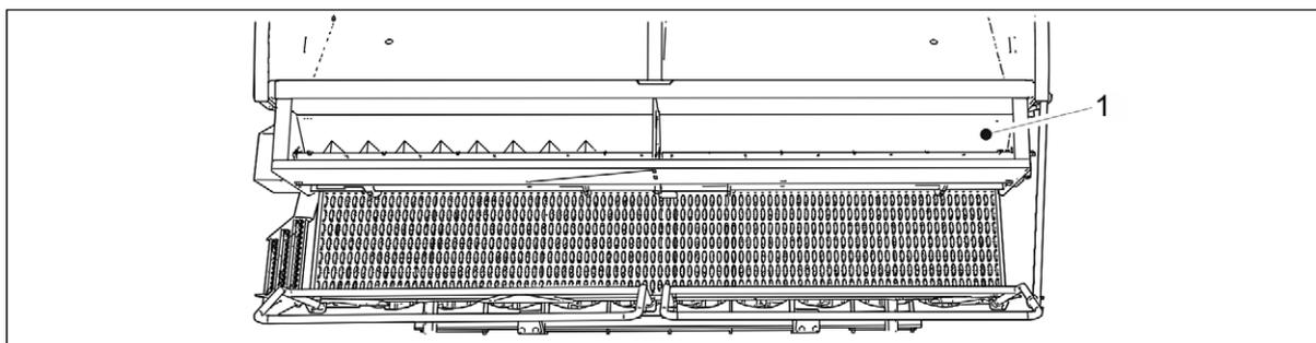
**Figure. 7.3.2. - 215. Cleaning of the small seed hopper**
