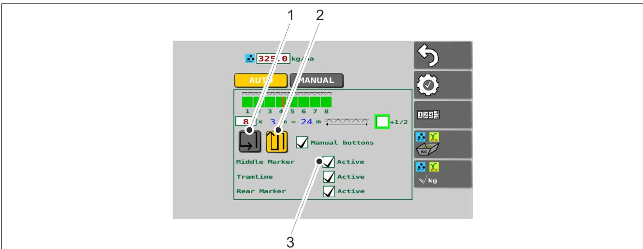
**Figure. 6.3.5. - 101. Selecting the middle markers and driving mode**
