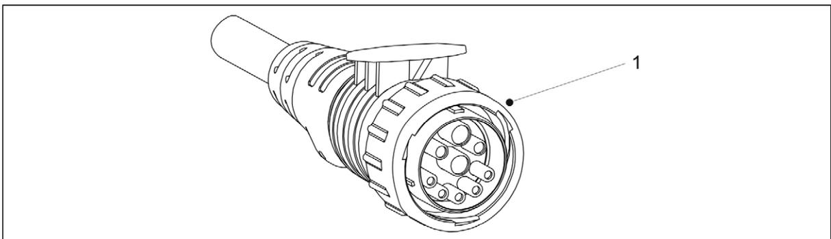
**Figure. 5.3. - 81. SeedPilot ISOBUS controller power cable**
