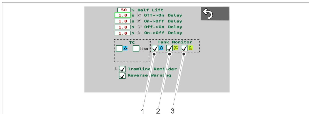
Figure. 6.3.8. - 106. Selecting hopper level sensors
