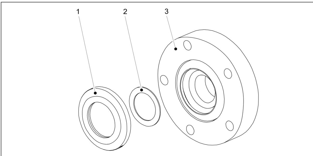
**Figure. 7.9.3.2. - 257. Bearing seal and shim**
