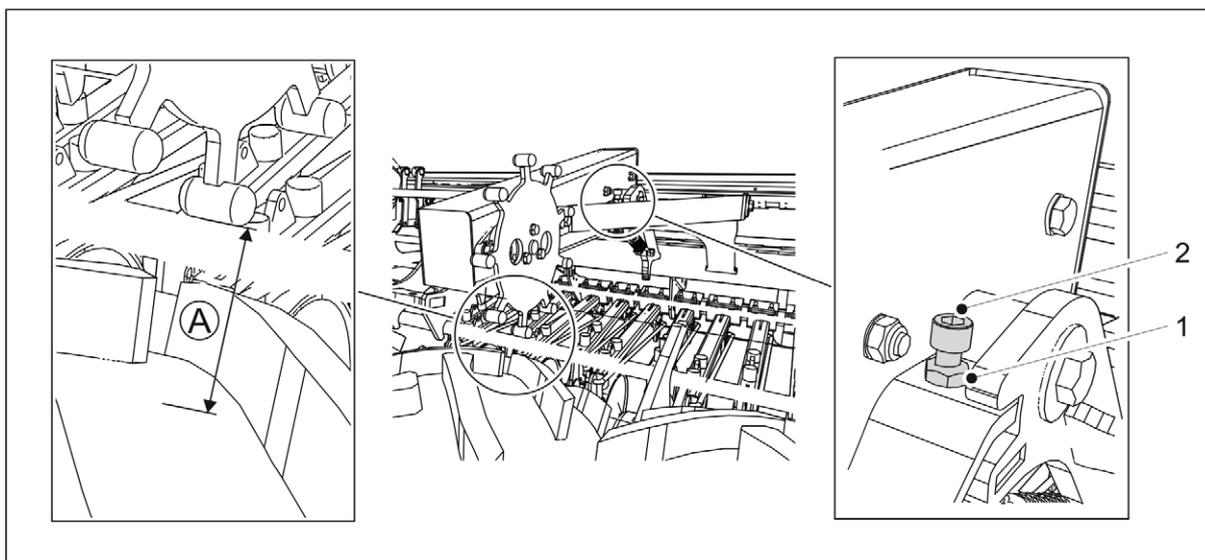
**Figure. 7.1.8. - 188. Inspecting the wheel drive clearance**
