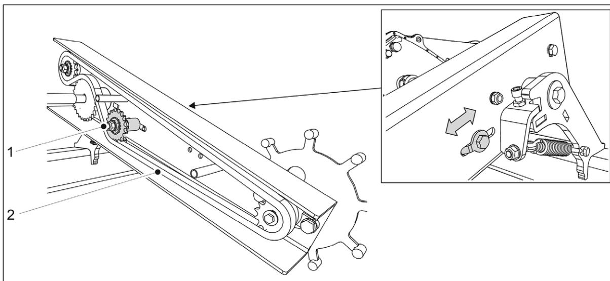
**Figure. 7.7.1. - 239. Tightening the wheel drive chain**
