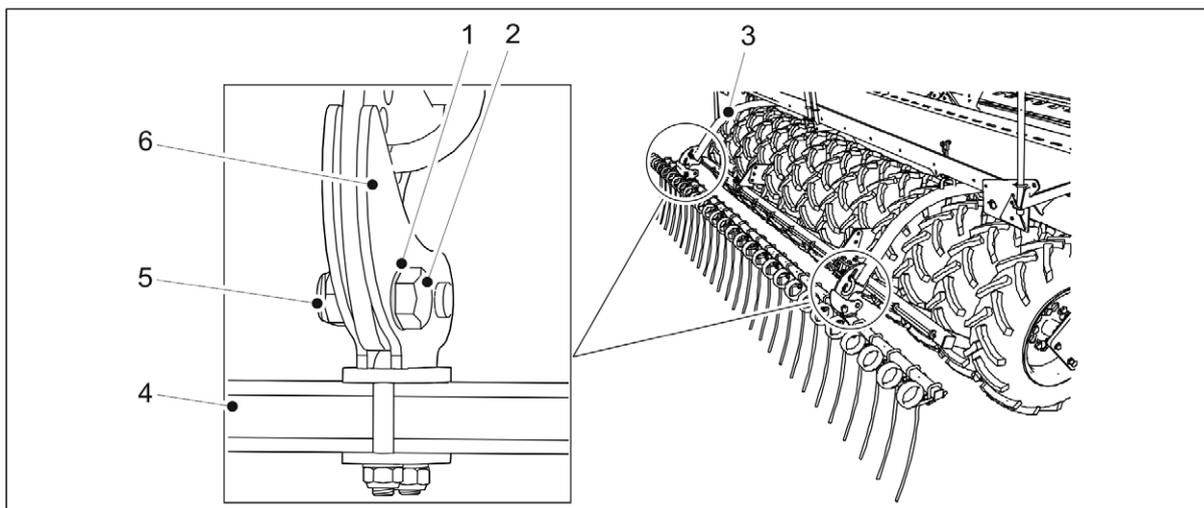
**Figure. 5.1.8. - 66. Mounting the rear harrow**
