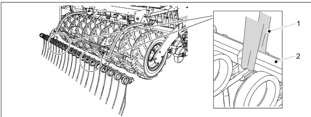
**Figure. 5.1.8. - 65. Lifting the rear harrow**
