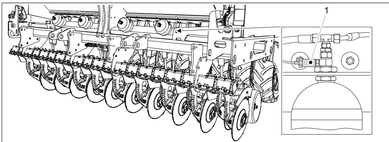
**Figure. 4.2.1.9. - 23. Coulter pressure sensor**
