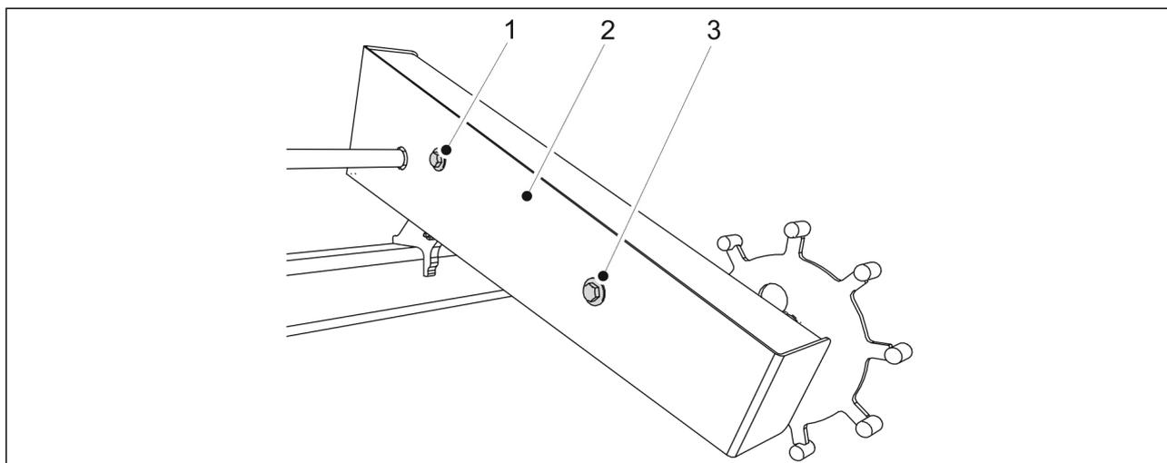
**Figure. 7.7.1. - 238. Opening the wheel drive housing**
