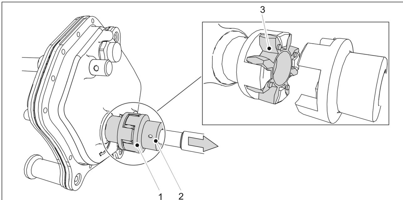
**Figure. 7.7.2.1. - 240. Dismounting the clutch rubber**
