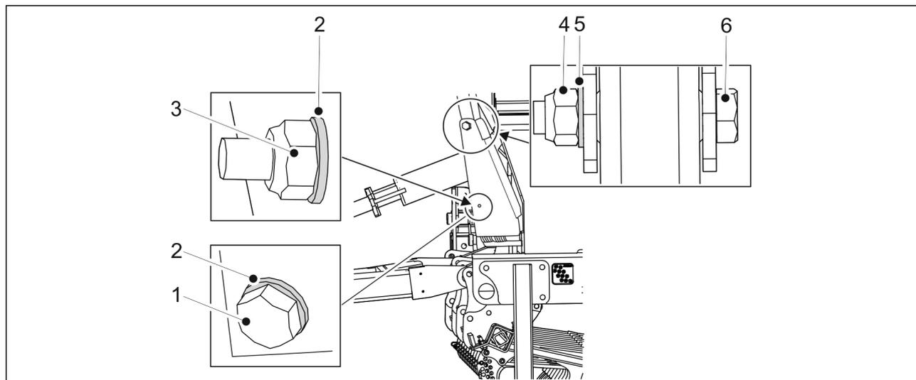
Figure. 5.1.5. - 60. Mounting the middle markers
