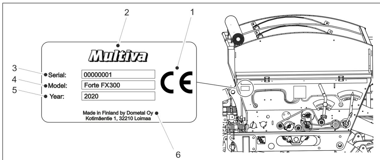
**Figure. 1.3. - 1. Location and details of the type plate**
