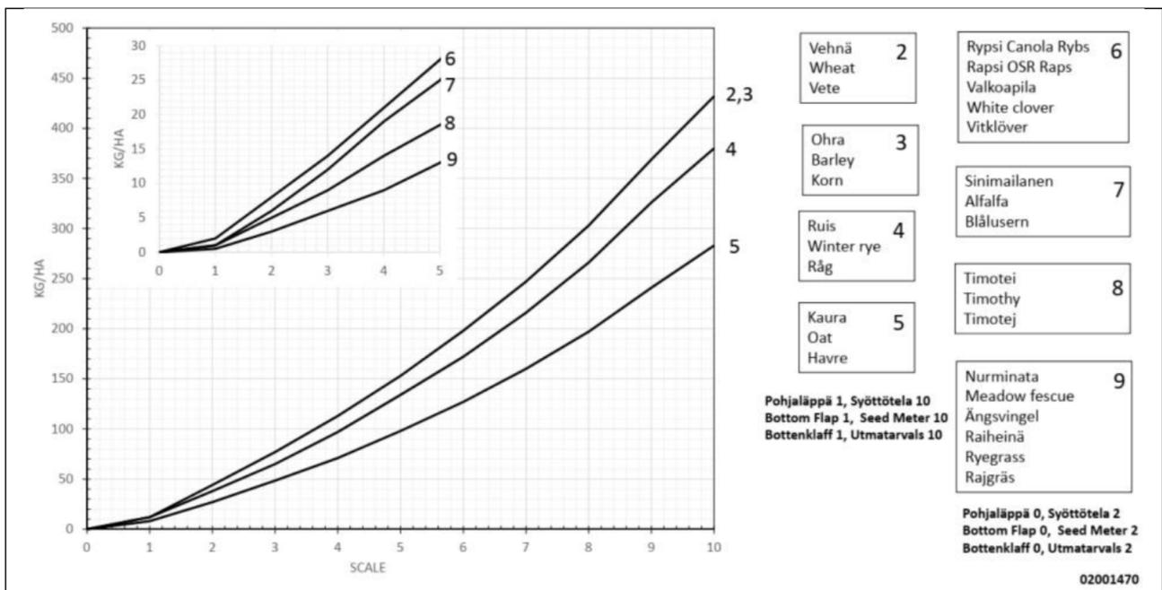
Figure. 6.5. - 116. Seeding table - seed and fertiliser gearbox 1
