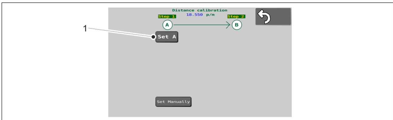
**Figure 7.10.2.1. - 263. Travel distance calibration 1**
