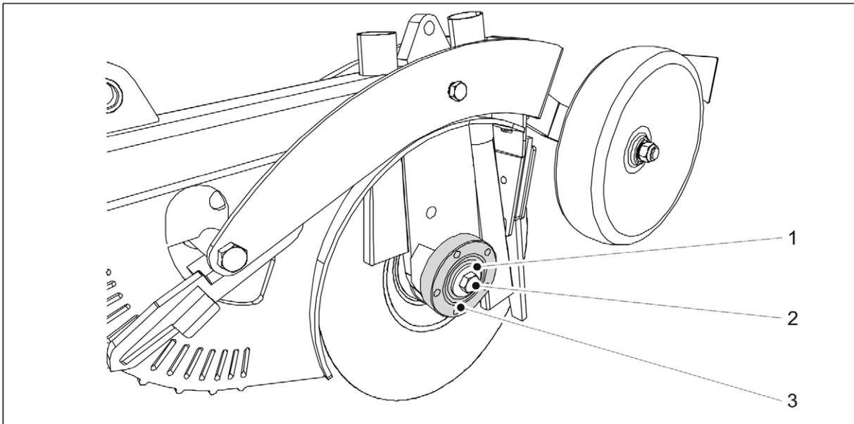
**Figure. 7.9.2.1. - 251. Detaching the bearing housing**
