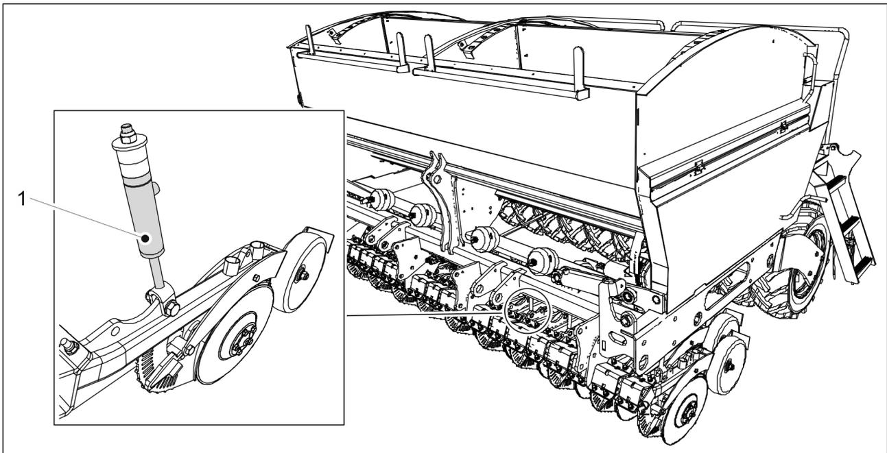
**Figure. 6.10. - 162. Adjusting the coulter pressure**
